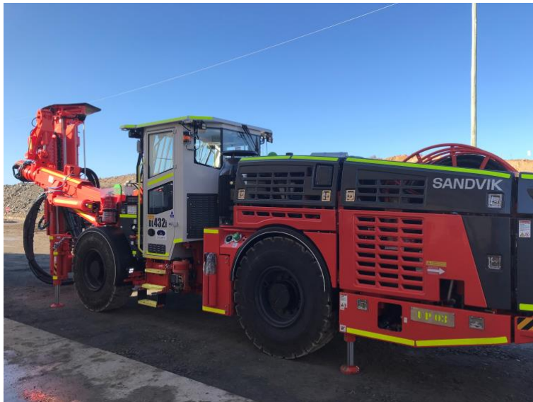
New Sandvik DD422i jumbo on site at Tomingley
