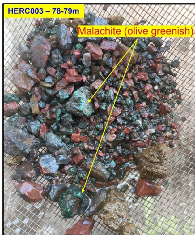
Photo 2: Reverse Circulation drill chips showing copper (malachite) in the oxide zone of drill hole HERC003.
