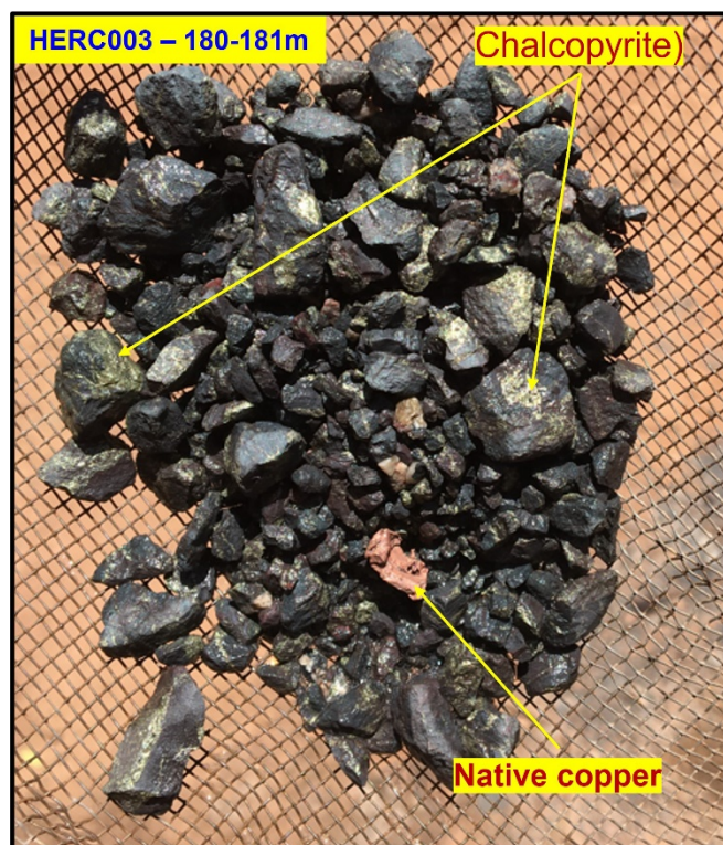
Photo 3: Reverse Circulation drill chips showing copper (chalcopryite) in the deeper primary of drill hole HERC003.
