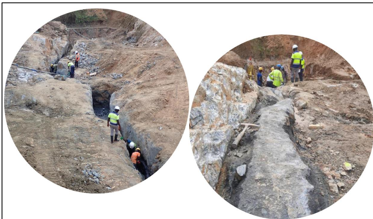
Figure 9: Bulk sampling of the Peyima kimberlite dyke
