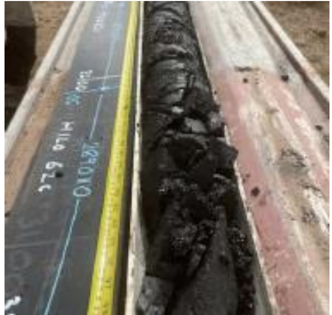
Figure 3: Core from Hole HIL054, twinned as HIL062C for coal quality analysis.
