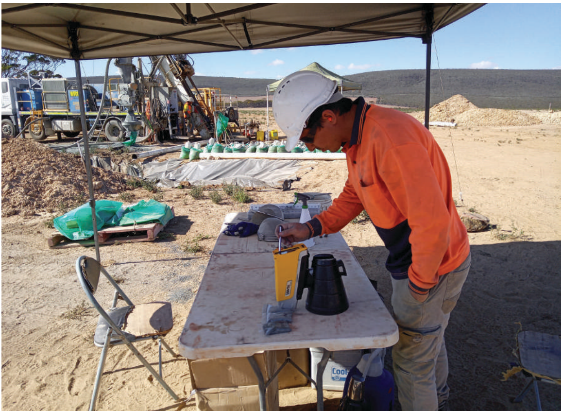
Testing samples using XRF
