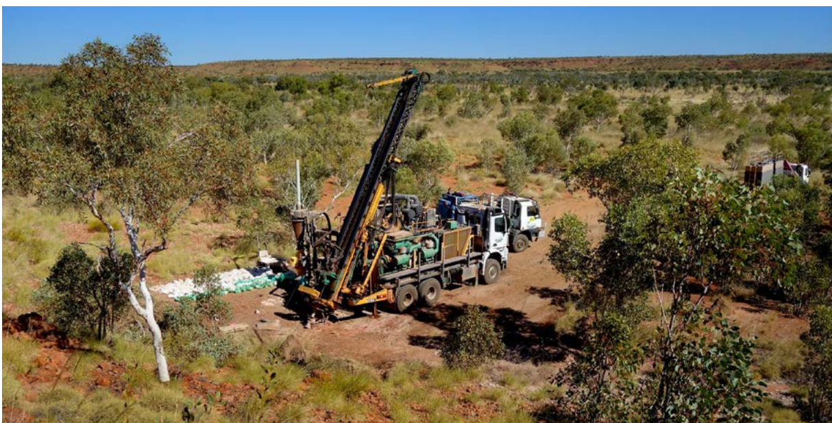
Figure 1: RC Drilling at Rockslider
