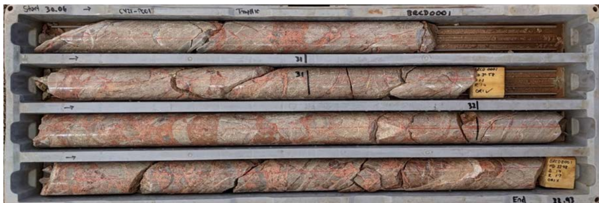
Figure 2. Cyclops Xenotime Breccia 30.06m to 32.93m down hole depth (Pink mineral = Xenotime)
