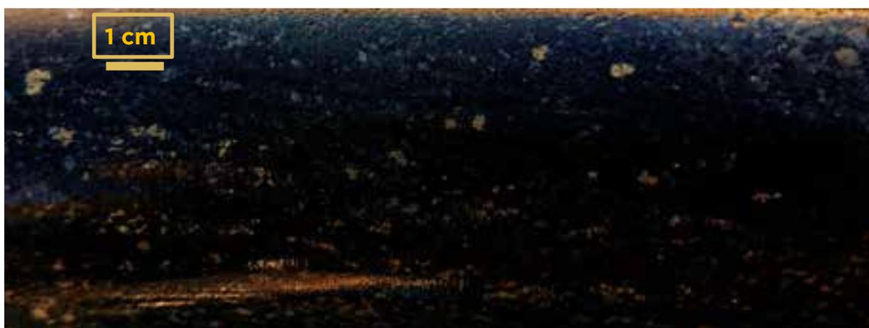
**Figure 1.19.** Extensive pyrite in layered gabbro. Note how the sulphide blebs which are up to 0.5 mm in dimension are intergrown with, and are an integral part of, the minerals within the gabbro. These textures are characteristic of magmatic sulphides and extend over a true thickness of about 100 m.
