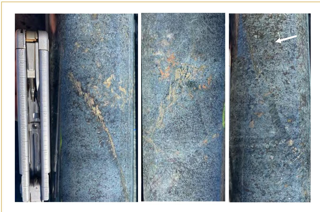
**Figure 1.18.** Photographs of diamond core from selected intervals from 95 m to 98 m down hole in RWIPT016. The photographs show disseminated to blebby to vein hosted sulphide mineralisation comprising pyrite-pyrrhotite-chalcopyrite (copper sulphide) and lesser pentlandite (nickel sulphide). Fine grained disseminated sulphide occurs in many places in this interval (see arrow for example)
