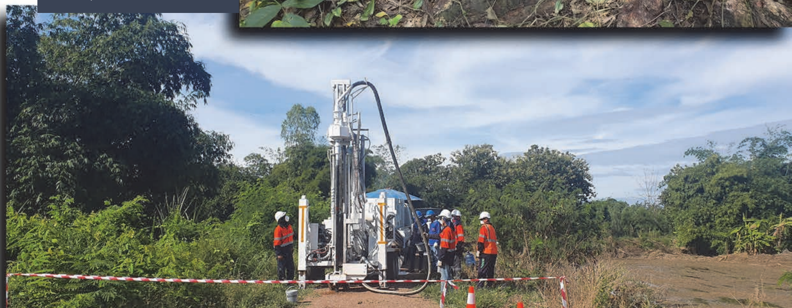
(Below). RAB Drilling in SPL 12/2563 in Wang Pong District, Phetchabun.
