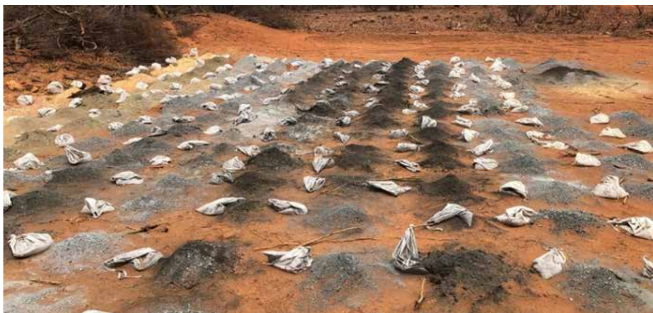
Ken's Bore RC Drill chips with broad massive sulphide zone
