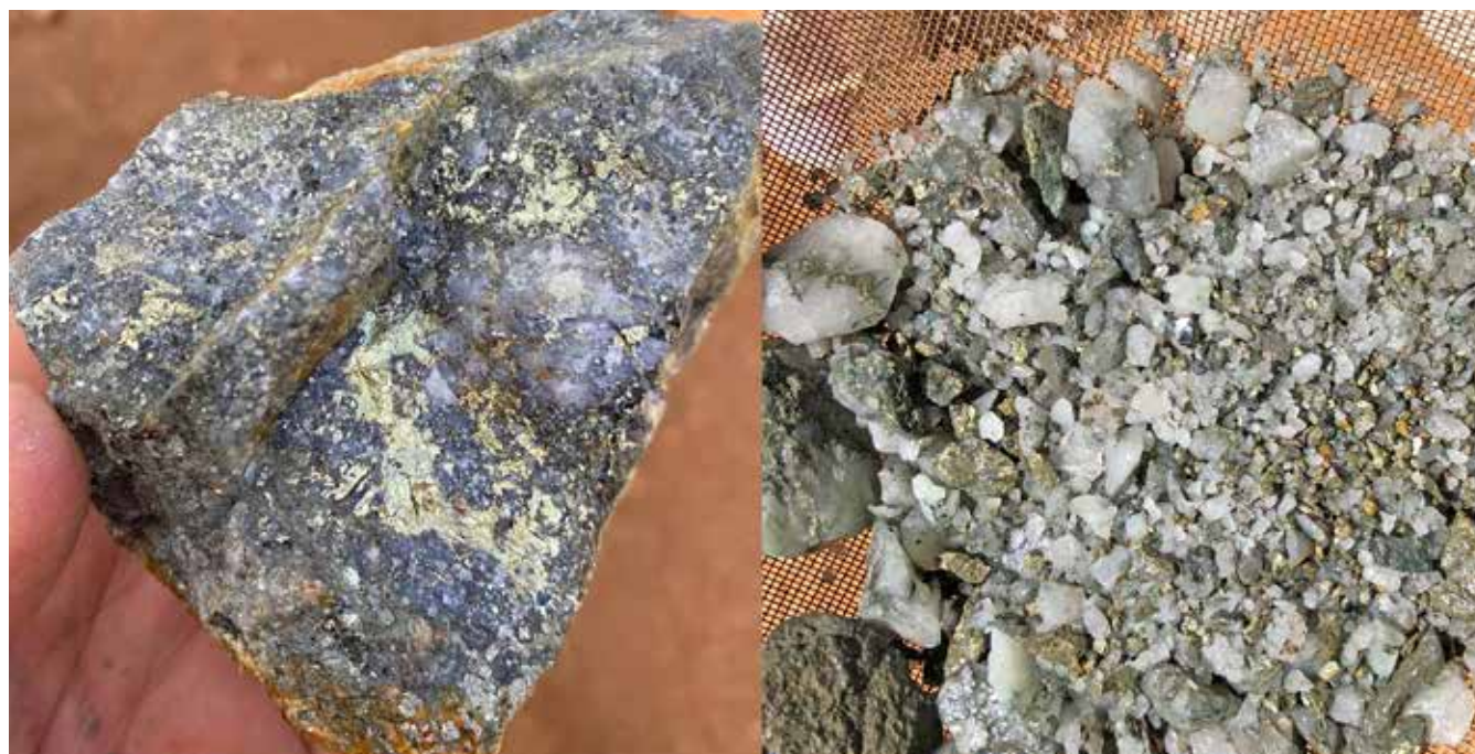
Comparison of quartz-sulphide mineralisation from Lake View surface dumps (left) with sieved chips from HMLVRC001, interval 44-45m assayed at 4.65% Cu and 0.52g/t Au (right) (See ASX announcement 22 June 2021)
