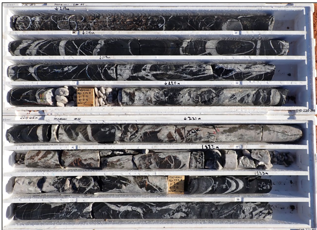
Figure 3: Core from PDD0001 showing quartz-carbonate veining and pyrite associated with the Grace/Bemm fault zone from 216.8m to 223.89m
