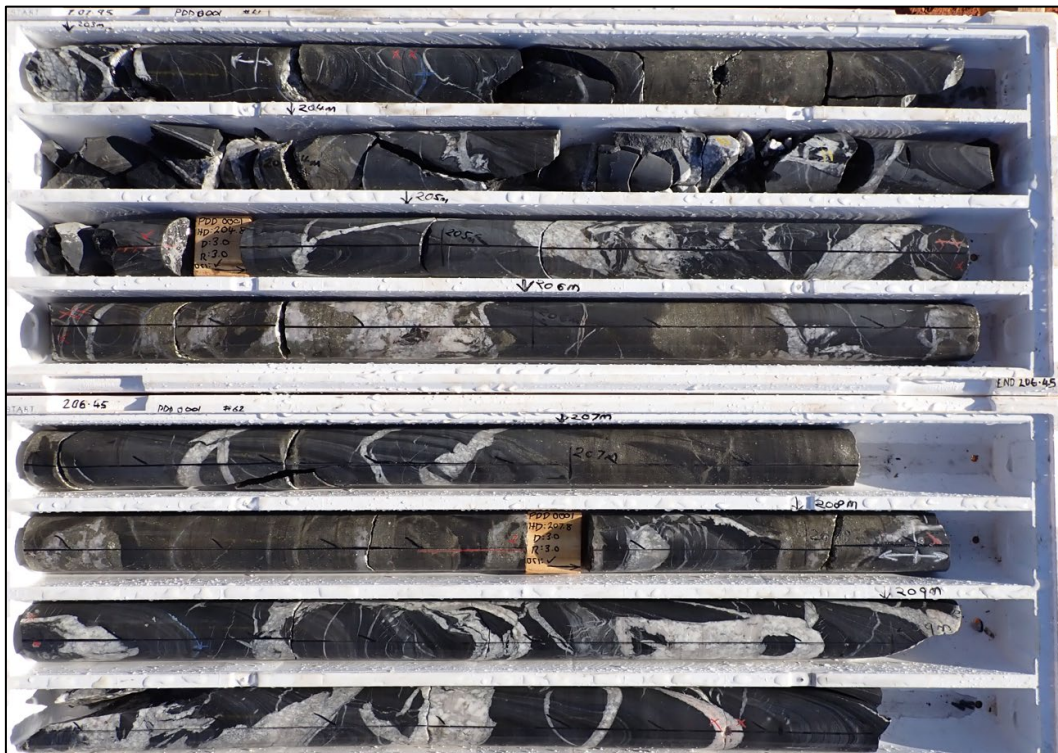
Figure 2: Core from PDD0001 showing quartz-carbonate veining and pyrite associated with the Grace/Bemm fault zone from 202.95m to 209.85m.
