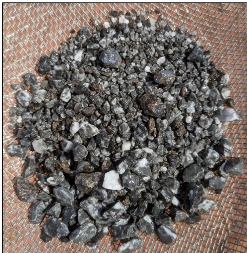
Figure 10: IQRC001 (137 to 138 metres). Sphalerite (red-brown-yellow) and galena (light grey) with associated carbonate veining within the Iroquois dolomite unit (dark grey). 12.7% Pb and 8.9% Zn
