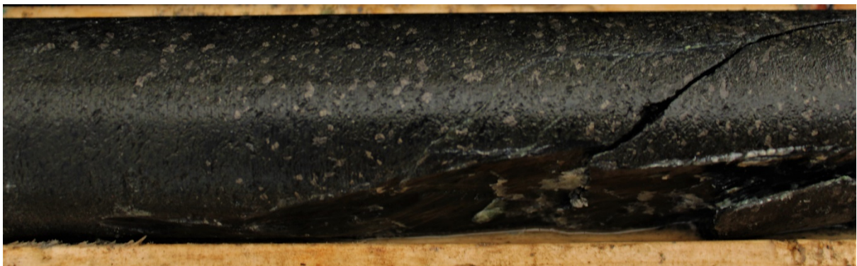
Figure 9: DDED21-059: Coarsely disseminated sulphide (pyrrhotite-pentlandite) 5% within medium grained peridotite from 180.5m
