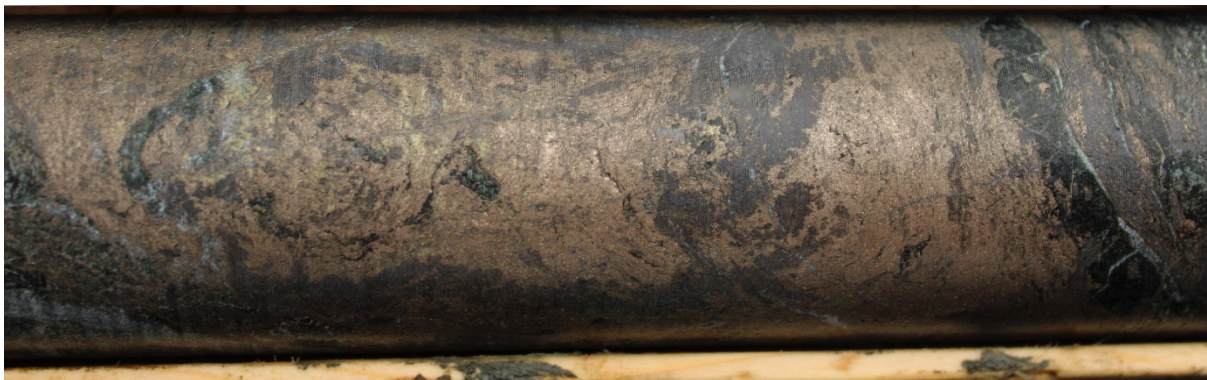
Figure 1: DDED21-059: semi-massive (pyrrhotite-pentlandite-chalcocopyrite) within fine grained sheared peridotite at contact with rhyolitic tuff at 54.5m (dry core)
