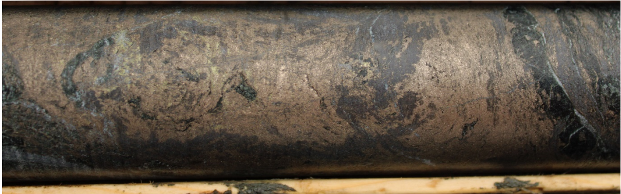
Figure 7: DDED21-059: semi-massive (pyrrhotite-pentlandite-chalcopyrite) within fine grained sheared peridotite at contact with rhyolitic tuff at 54.5m (dry core)
