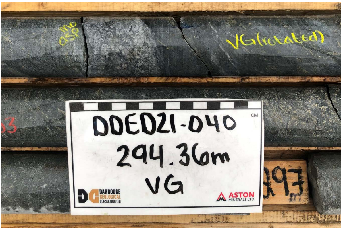
Figure 14: Visible Gold Within Quartz-Carbonate Vein Associated with Arsenopyrite & Molybdenum
