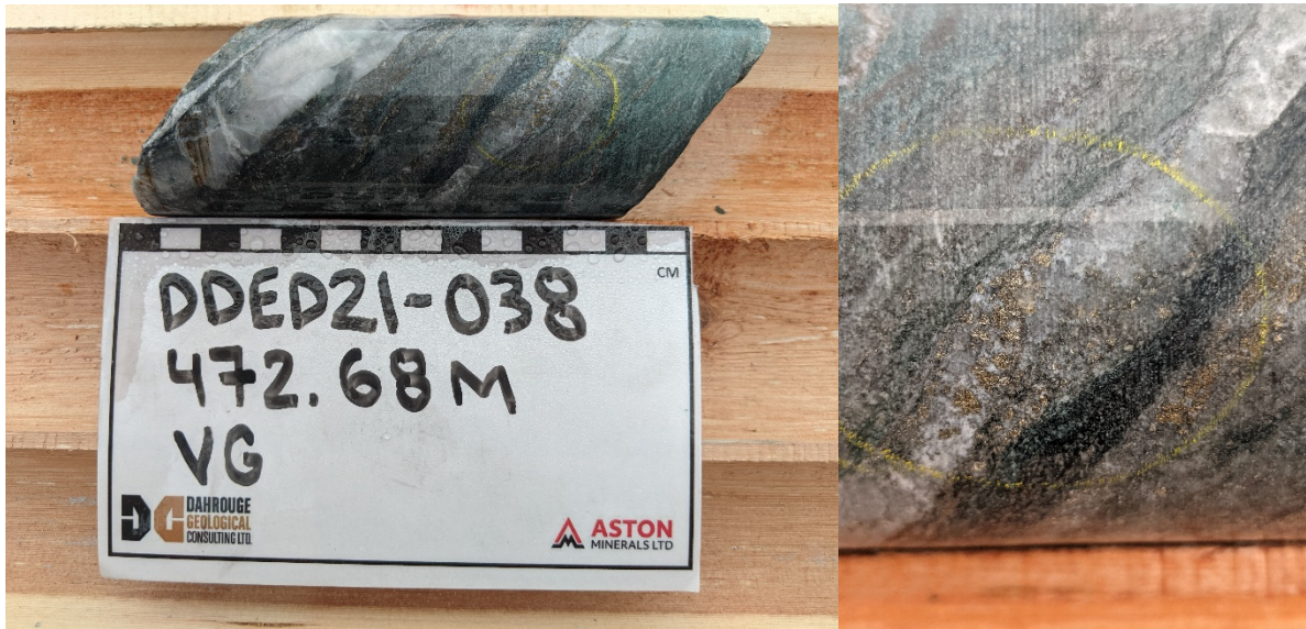
Figure 13: Visible Gold Within Laminated Quartz Vein, Host Basalt Contains Locally 8% Pervasive Fine Grain & Blebby Pyrrhotite
