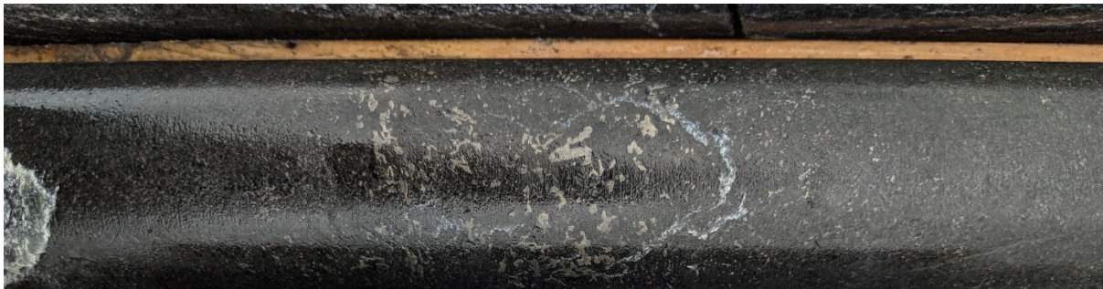
Figure 113: DDED21-059: Fine disseminated to medium grained blebby (pyrrhotite-pentlandite) 5% within peridotite from 256m
