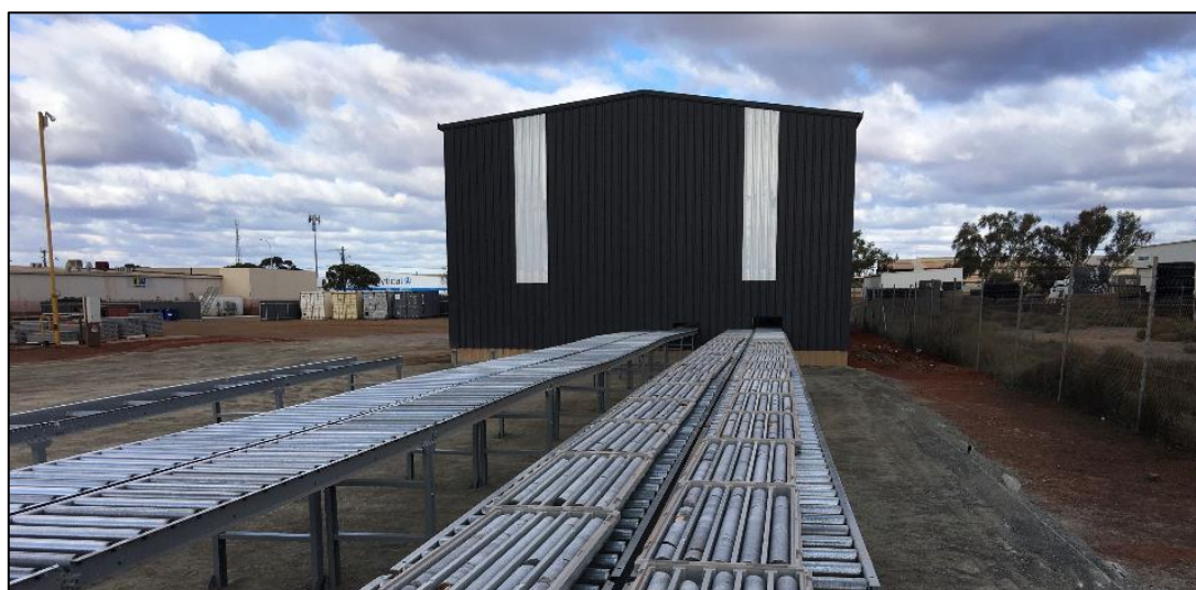
Figure 17: Roller racking at Iceni's Kalgoorlie core yard. The racks can hold 600m of NQ core, which is fed to twin Almonte diamond core saws within the shed.
