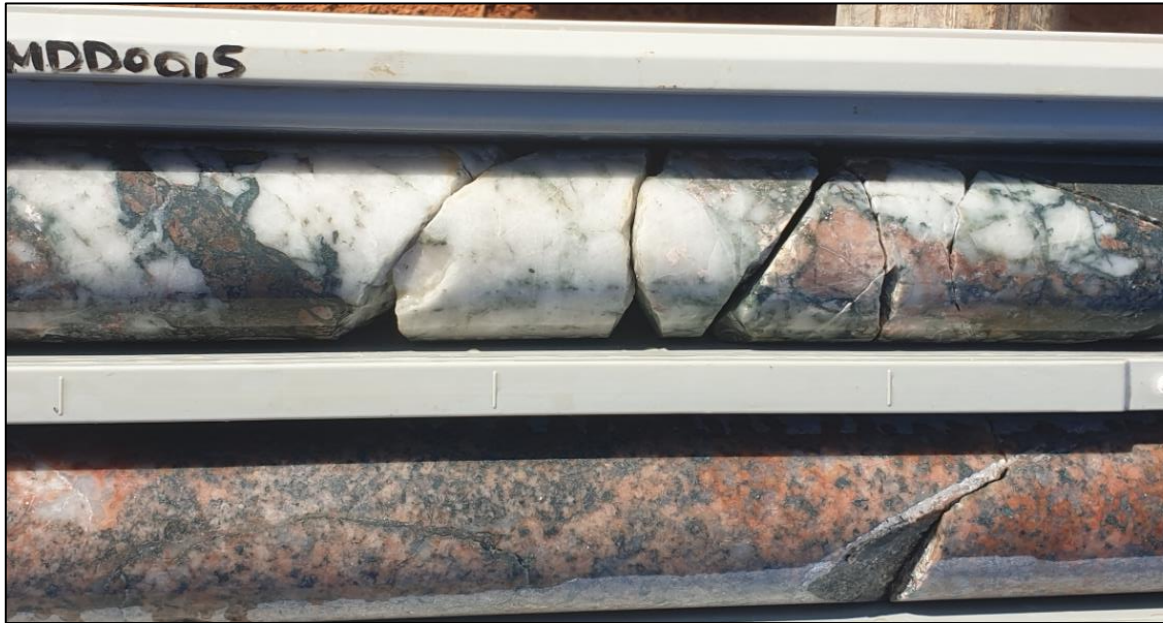
Figure 13: Strongly hematite, silica and sulphide altered drill core at ~210m in FMDD0015.
