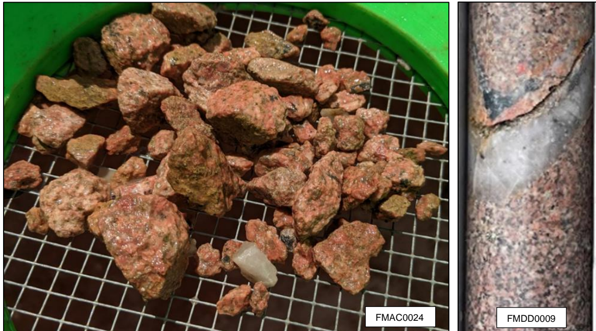
Figure 5: Early success in the AC drilling at Deep Well in hole FMAC0024. The AC drilling has intersected quartz veining and associated hematite alteration with weathered sulphides (left). This is identical to intersections from the focussed diamond drilling (right), which is located several hundred metres to the south.
