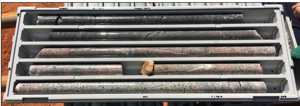
Figure 12: FMDD0012 at ~95m, showing an intermediate porphyry cutting the Danjo Granite. The porphyry contains disseminated sulphides throughout. The granite displays brecciation and hosts several quartz veins. Overall, the rock mass has seen an enormous amount of hydrothermal fluid that has modified significant volumes of rock. This is a process that can form large gold deposits.
