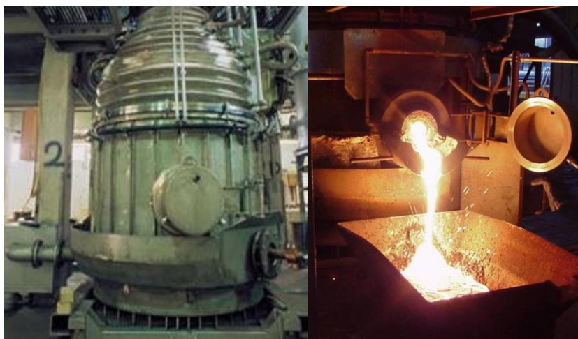
Figure 5 Close-up of the furnace (left) and pouring of slag after magnesium metal was extracted (right)
