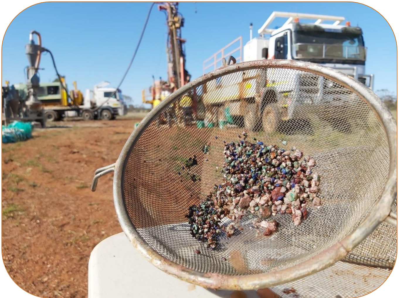
Figure 3 - Copper oxide mineralisation; azurite (blue) and malachite (green) in CORC0140 at 34 metres
