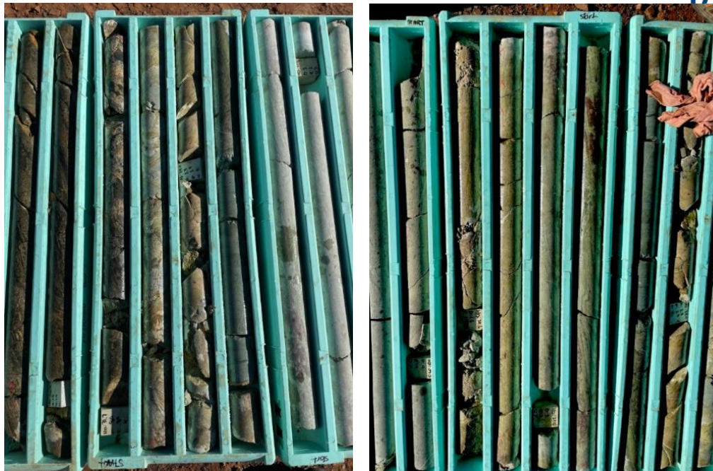
Figure 12. MCDD004 (left ) 30-35m biotite altered carbonate breccia with hydrothermal alteration, including sericite and sodic alteration ; and (right) – 37 – 43m strongly serpentinized carbonate breccia with magnetite and hematite alteration.
