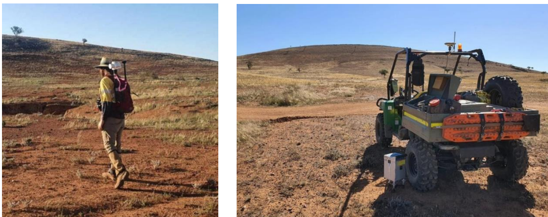
Figure 13. Ground-based Magnetics (left) and Gravity (right) Programs currently underway at Mt Craig Copper project.
