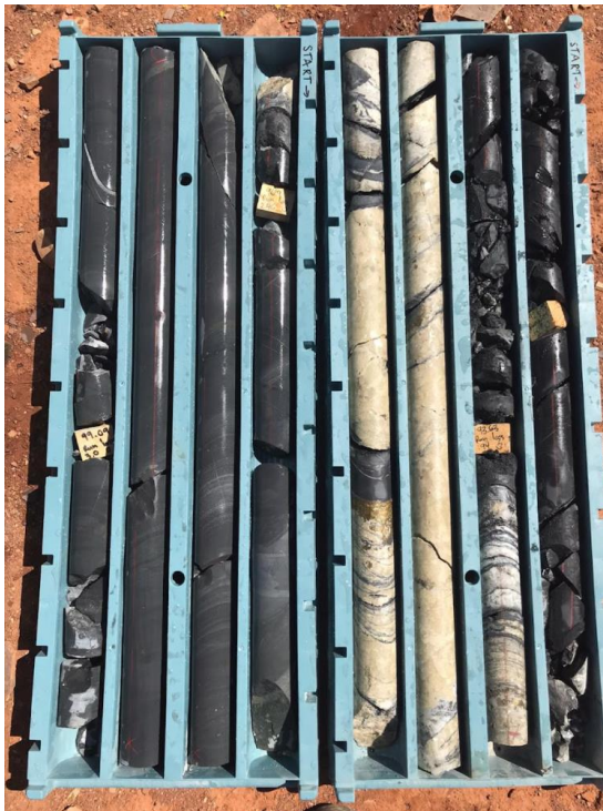
Figure 1. Primary Ore Zone at Worrumba-19, Comprised of Blebby to Semi-Massive Chalcopyrite in Massive Dolomite, and Disseminated Chalcopyrite in Black Shale at the Base of the Tindelpina Shale Member (Drillhole WCDD001).
