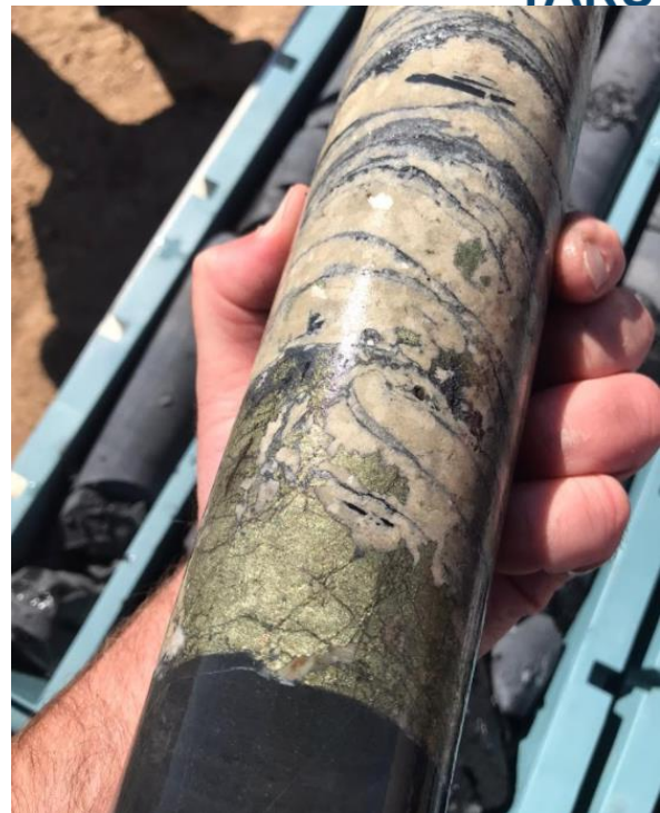
Figure 1. Primary Ore Zone at Worrumba-19, Comprised of Blebby to Semi-Massive Chalcopyrite in Massive Dolomite, and Disseminated Chalcopyrite in Black Shale at the Base of the Tindelpina Shale Member (Drillhole WCDD001).
