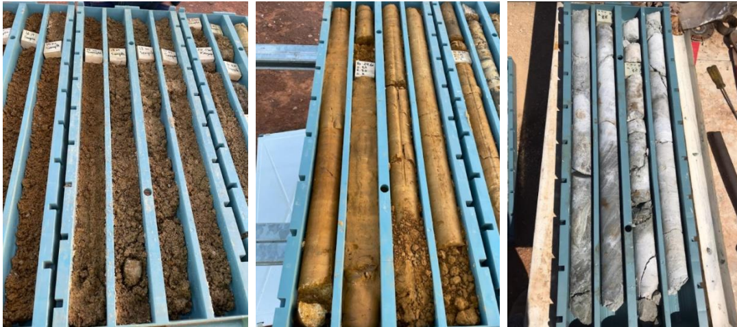
Figure 9. (left) Near-surface core from MCDD003, showing heavily brecciated and oxidised metasediments containing Zinc, Lithium and REE mineralisation identified from recent RC drilling (5-17m in image)), (centre) more competent oxidised sedimentary breccia (~22-26m in photo); and (right) brecciated crystalline marble unit contacting on brecciated mafic-ultramafic intrusion.
