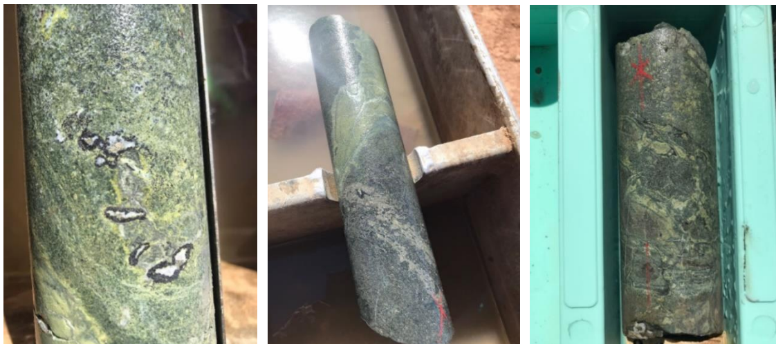
Figure 11. MCDD004 ( left) Biotite-calcite-magnetite-serpentine-pyrite alteration at approximately 31m; (centre) magnetite and pyrite (+ minor arsenopyrite + chalcopyrite) alteration ~45m; and (right) chloritized ultramafic on the margin of the diapir at approximately 26m.
