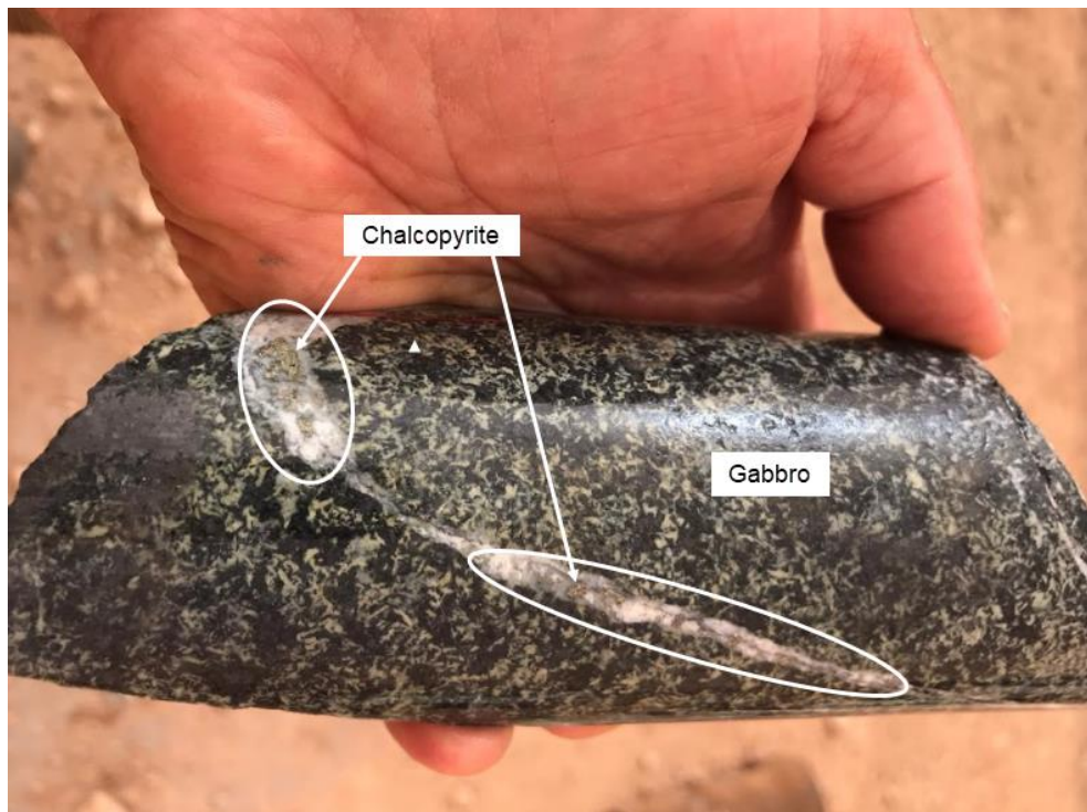
Figure 10. MCDD004 Chalcopyrite Mineralisation within calcite veining in Gabbro at approximately 149m.
