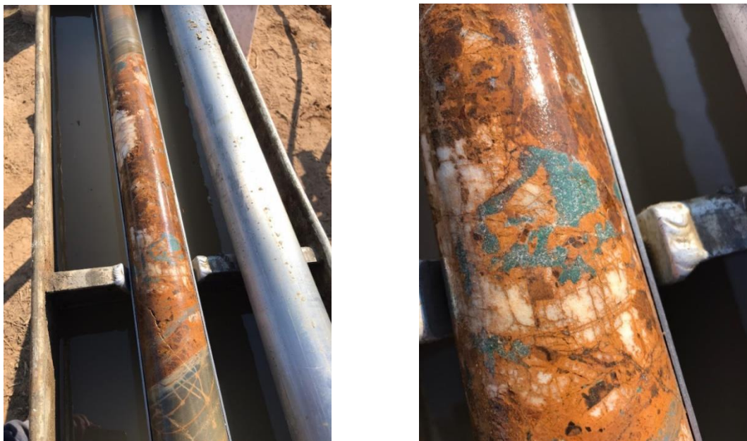
Figure 4. The Oxide Ore Zone at Worrumba 21, Hosted within Lower Tapley Hill Formation Shales, showing Malachite Mineralisation within Siderite-Ankerite and Dolomite Matrix.
