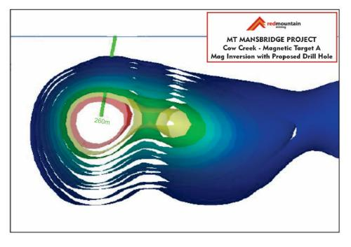
Figure 5 – Mag Target A – Inversion Slice and Planned Drill Hole
