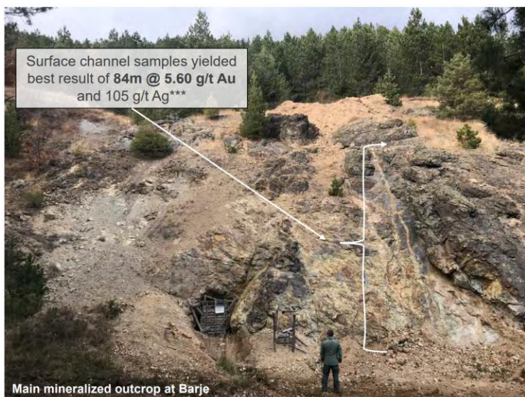
Figure 3, 4 and 5: Exploration undertaken at the Tlaminio Gold Project. Figure 3 (left) - channel sampling at the main mineralised outcrop at Barje (Tlaminio Project); Figure 4 (right, top) - core sample from drilling in hole BAR010; and Figure 5 (right, bottom) - core sample from drilling in hole BAR013
