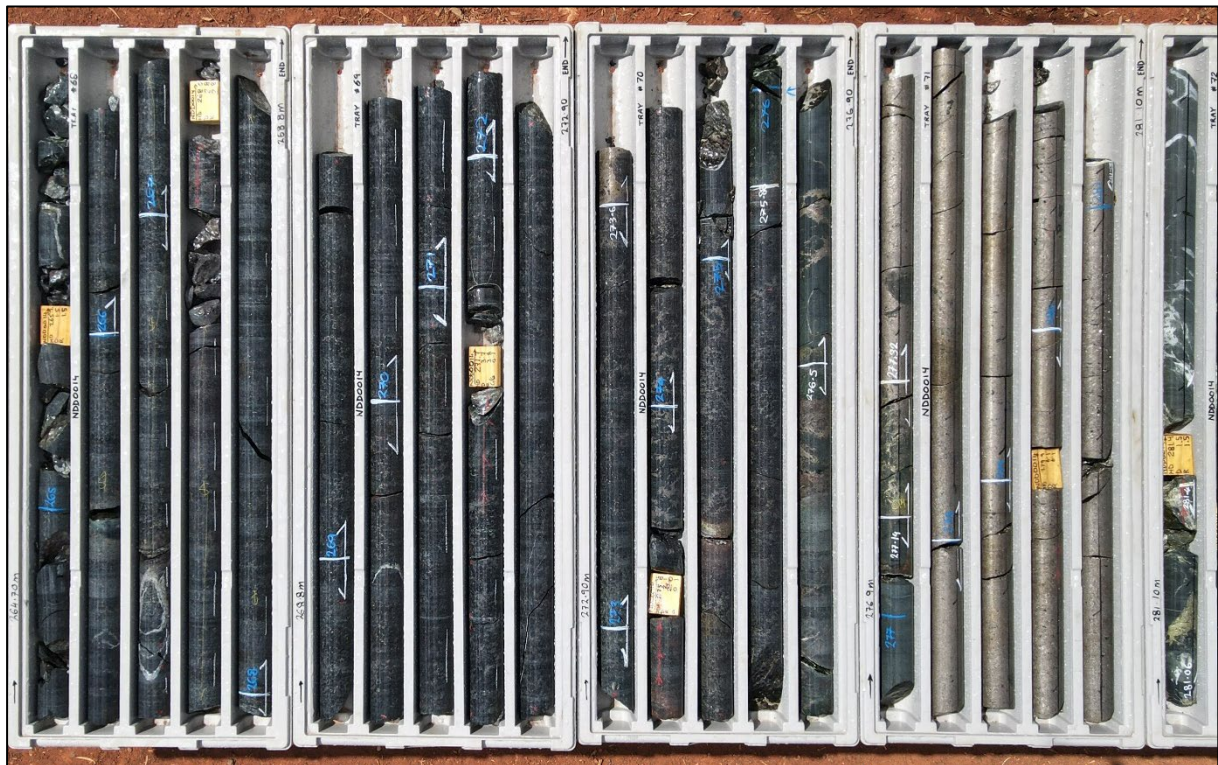
Figure 1. Massive sulphides intersected by NDD0014 in footwall metabasalts left shot, with a broad zone of heavy disseminated sulphide in ultramafics right shot.
