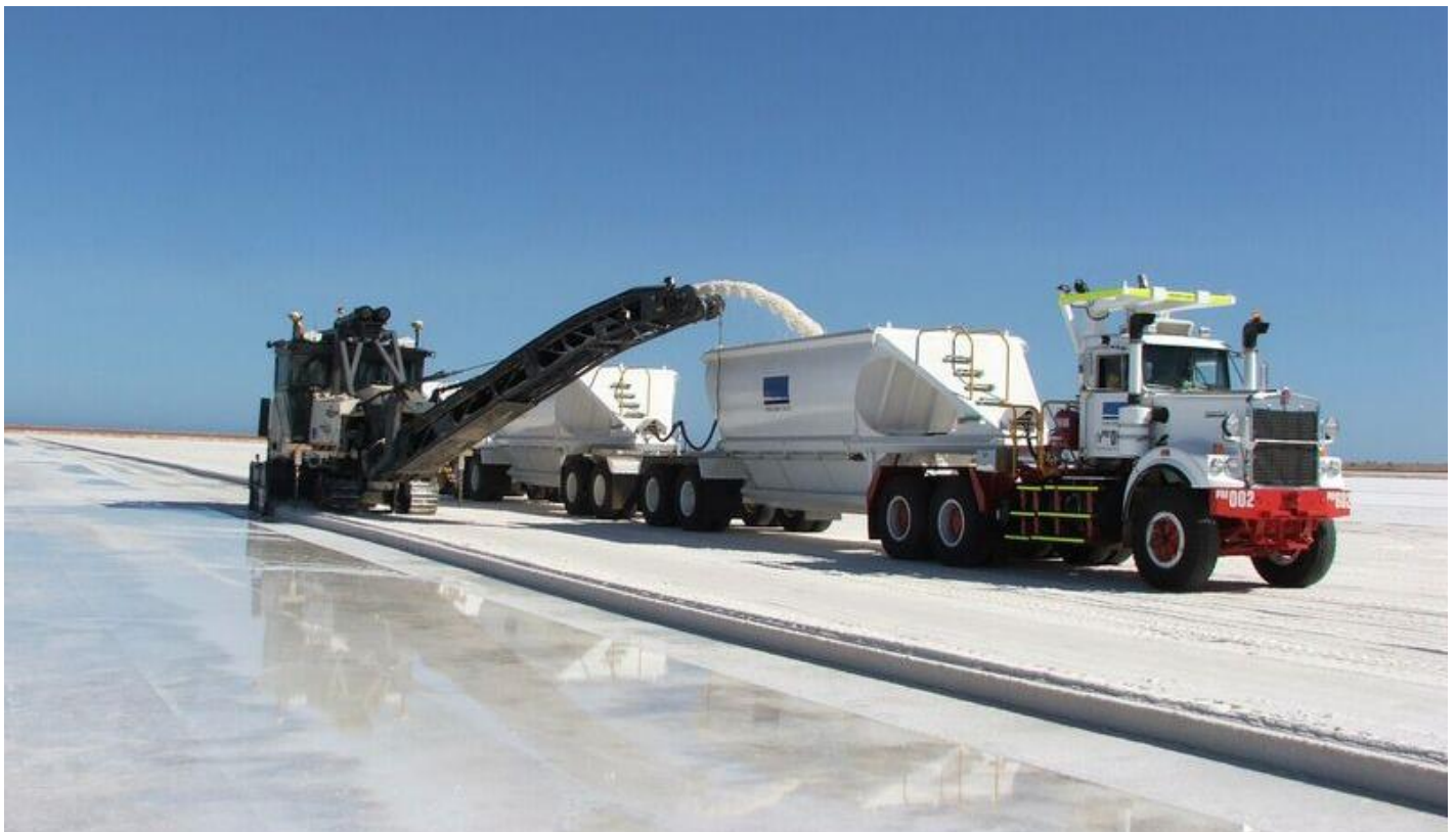
Figure 5: Typical Harvesting Method - A Wirtgen 2200SM Loading a B-Double Haul Truck
