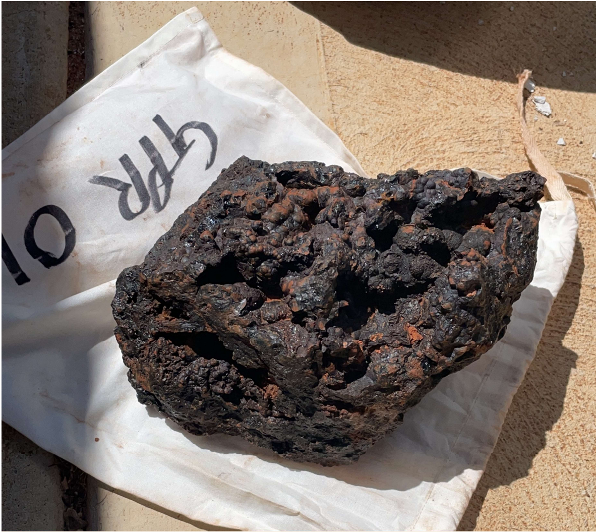
Figure 3. Rock chip sample GPR010 exhibiting botryoidal banding of potential Mn oxides and hydrous Fe oxides, such as goethite (>80% total rock mass, based on initial visual inspection) which are common features of Yangibana style ironstones. Note for scale, Calico sample bag is 27cm wide.
