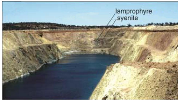
Figure 9: Syenite and lamprophyre are exposed in the Butcher Well open pit within the Laverton District (after Witt 2018).
