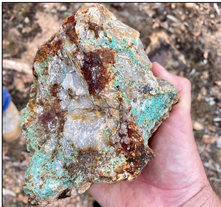
Figure 1. Quartz veining, weathering sulphide and malachite stain on fractures in rock chip sample from Gagarin (Sample GG013: 4.31% Cu, 0.45 g/t Au, 3.01 g/t Ag, 414 ppm Mo)
