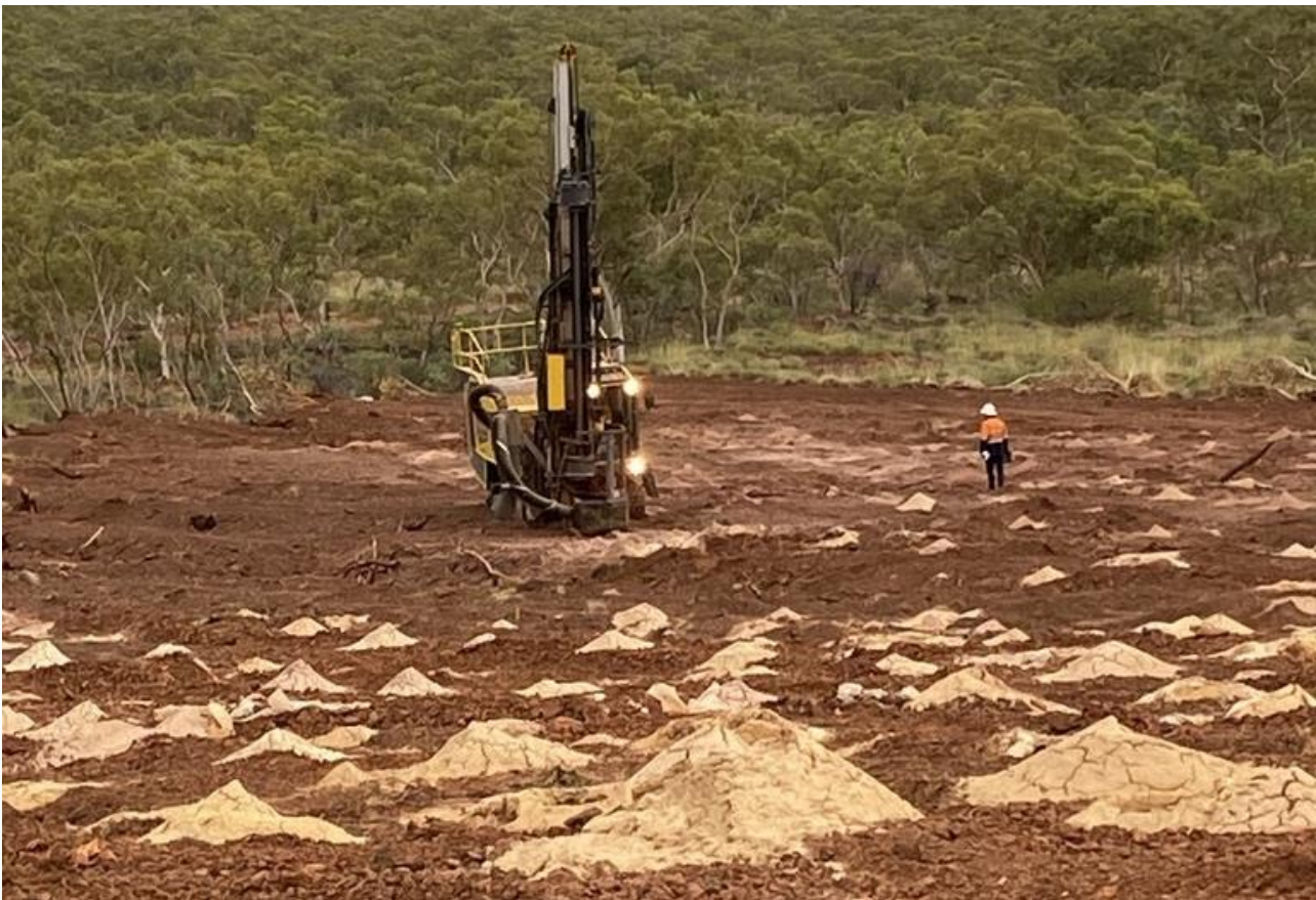
Figure 4. Drilling the first blasthole pattern at Anthill east pit.
