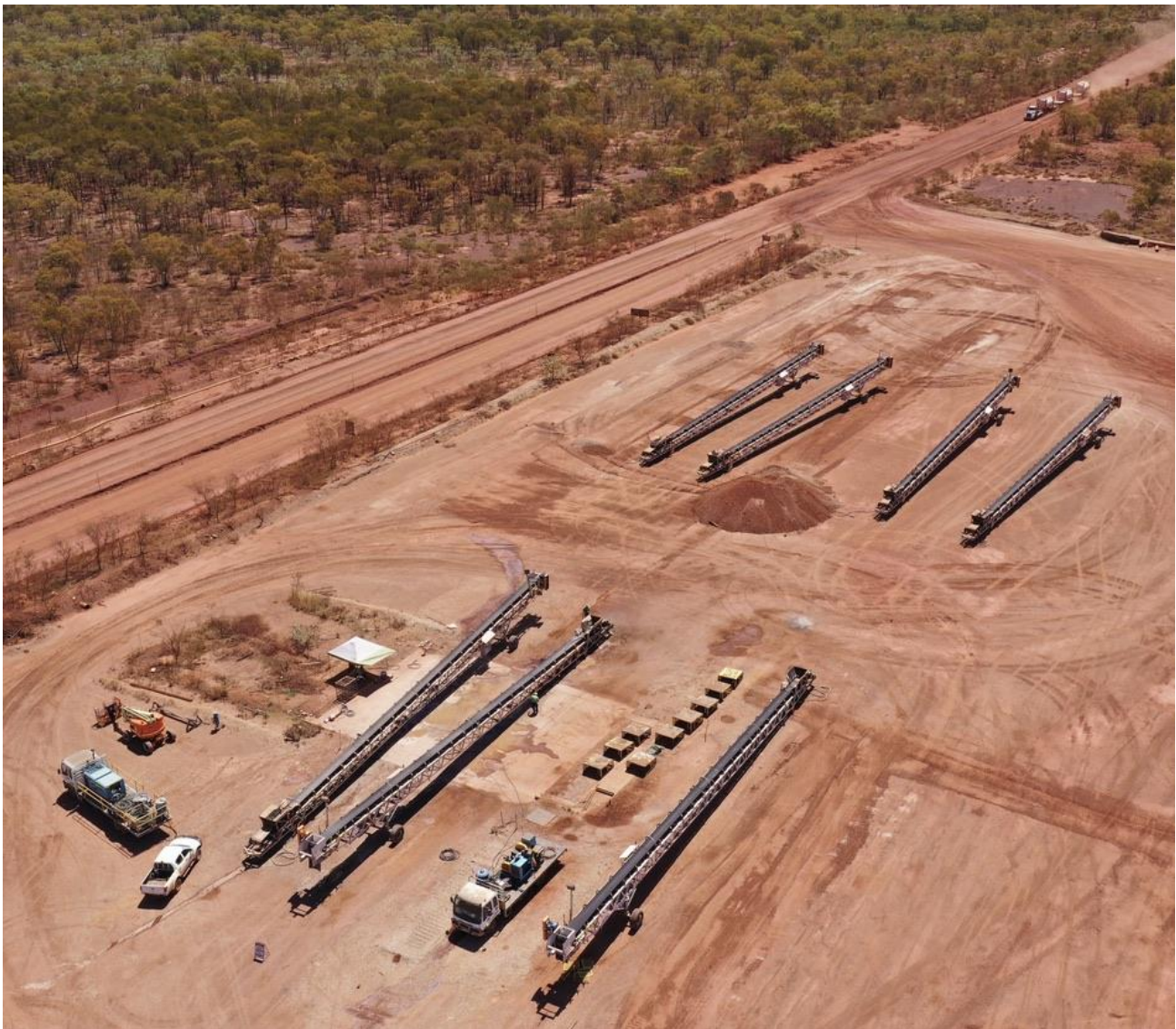
Figure 5. Stacking Conveyors at Mt Kelly being refurbished.
