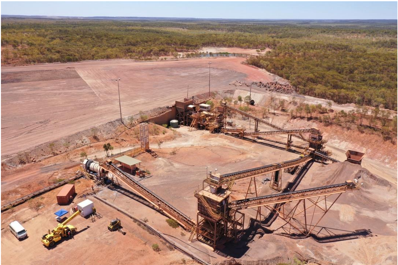
Figure 6. ROM pad in the background with feed bin, jaw, secondary crusher and screen house. Agglomerator on the front left of image feeds the conveyor to the heap leach pad.
