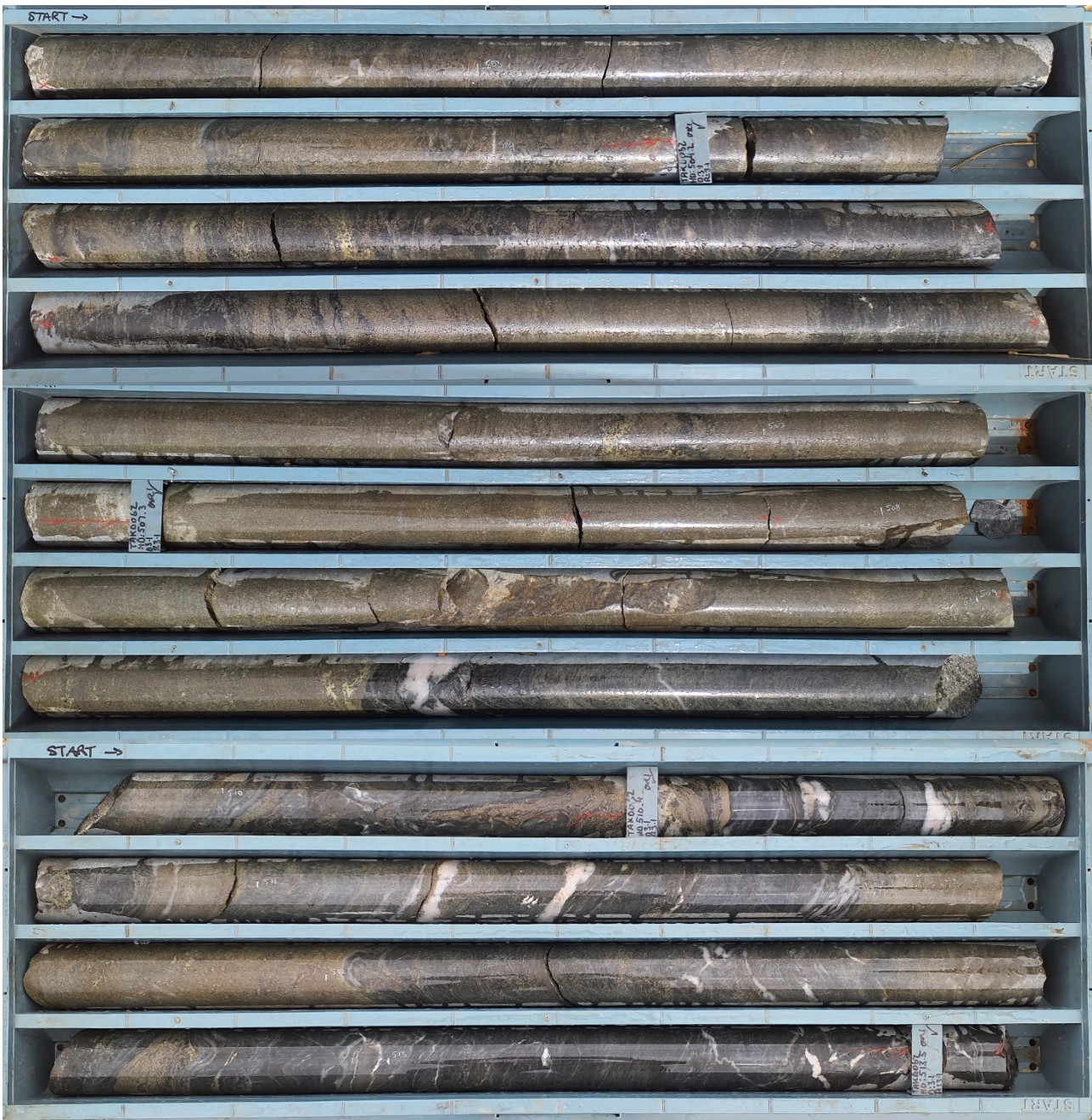
Figure 2 – Composite image of drill core through the banded and massive sulphide (dull yellow to bright yellow) intersection within drill hole TAKD062.
