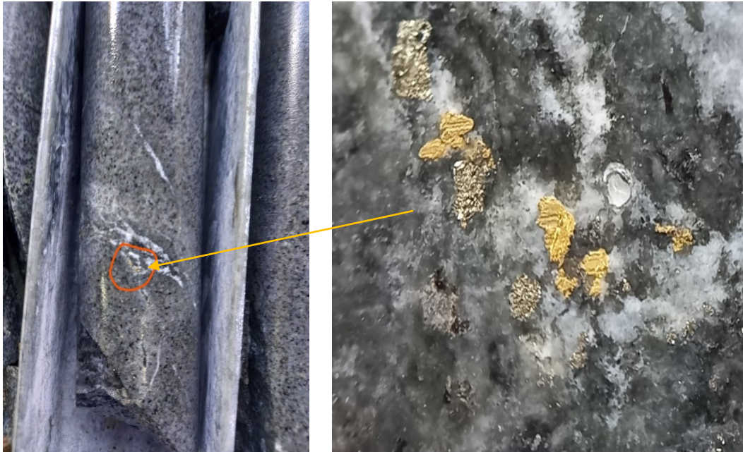
Figure 3: Photo of a portion of uncut drill core from TUDDH544W2, showing coarse visible gold and pyrite. This 30cm sample returned 112 g/t Au from 631.1-631.4m.
