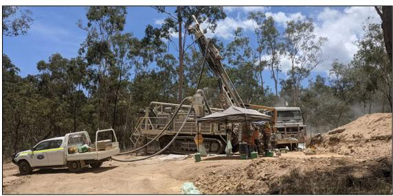
Figure 1. RC drilling at Big Hans
