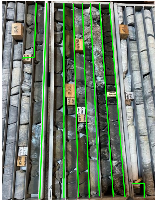
Figure 1: High grade copper chalcocite and chalcopyrite sulphide intersection GSQ core library historic drill hole DMD11 1
