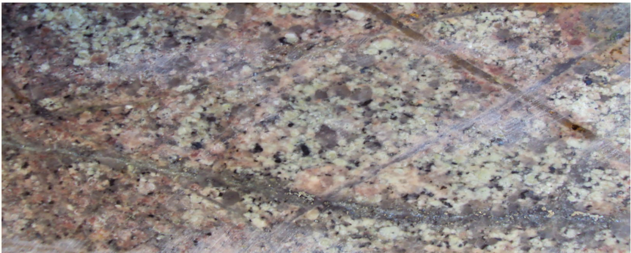
Figure 2: Copper Wolf core showing vein stockwork from hole CC-1A with classic multi-stage porphyry style alteration and Cu-Mo sulphide mineralisation (photo dated 13 th May 2009, depth ~611 m, width of photo ~ 6 cm).
