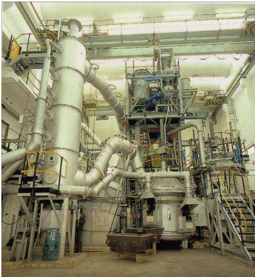
Figure 4 Magnesium plant which produced pure Winchester Mg - condenser (left), arc furnace (right)
