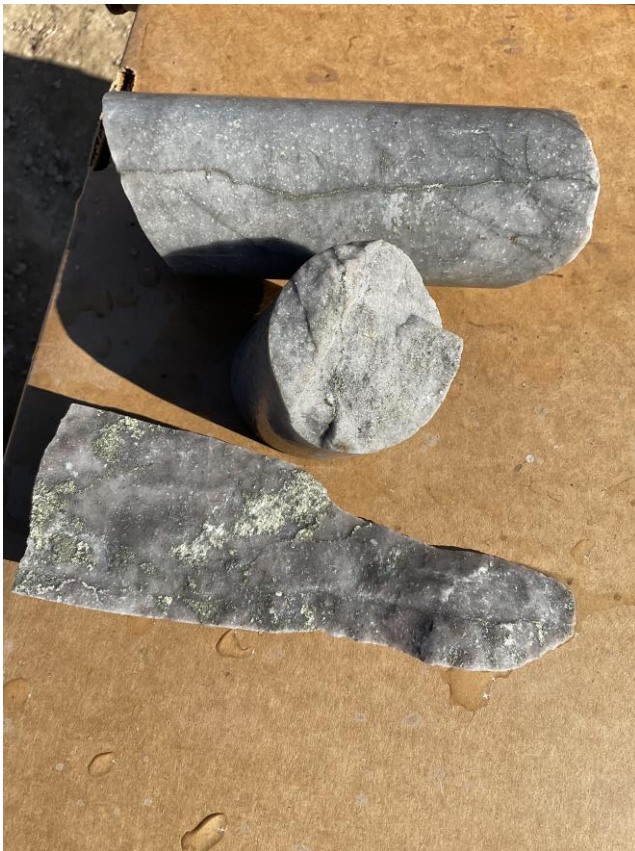
Figure 1: 7DD21-003 @ 45m: Porphyry with extensive fine-grained silica and potassic alteration; 2-4% disseminated pyrite plus stockworks with pyrite > molybdenite > chalcopyrite.
