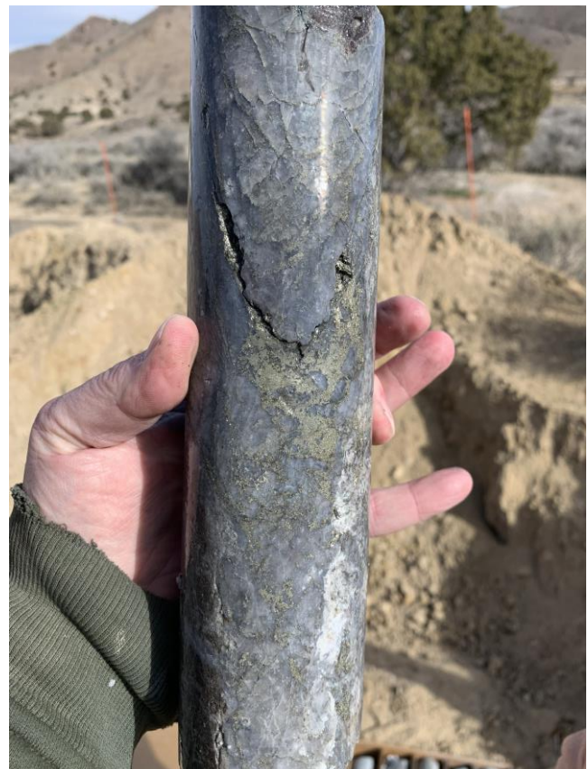
Figure 2: 7DD21-003 @ 488m: Strongly altered diorite and porphyry; 7-10% disseminated and fracture controlled sulphide with variable vein intensity; pyrite > molybdenite.
