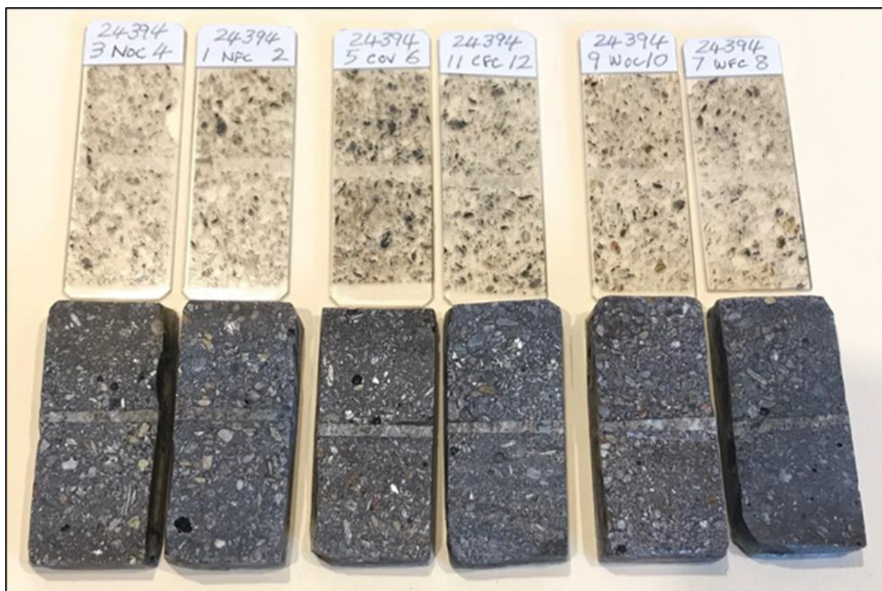
Figure 10: Variability composites prepared for thin section manufacture, and final thin sections
