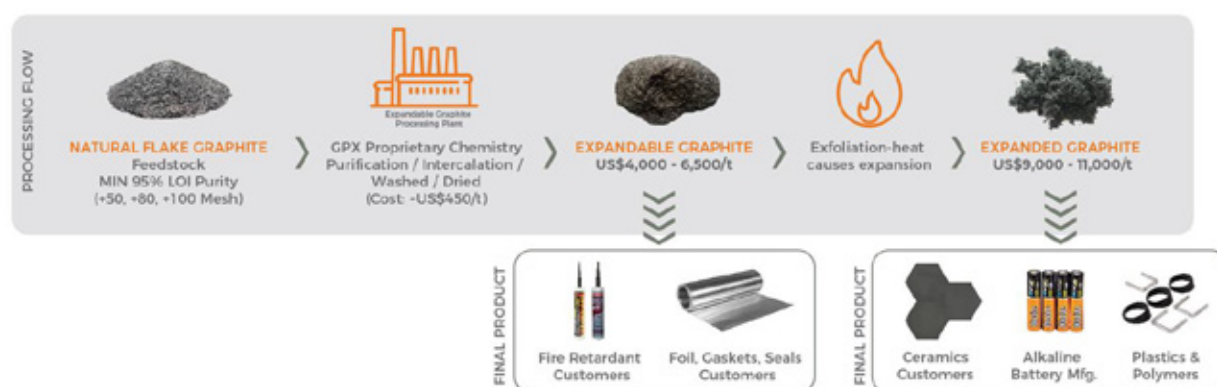
Figure 7: Process flow chart for expandable graphite and expanded graphite
