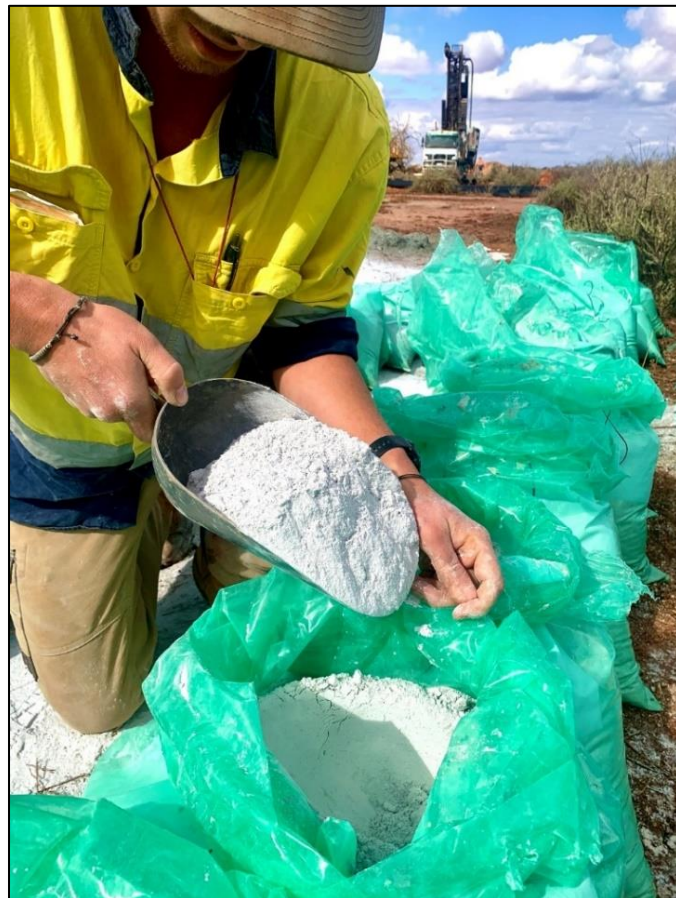
Figure 1; White Spodumene rich pegmatites in RC samples drilled from IDRC081 126m at the Mt Ida Project
