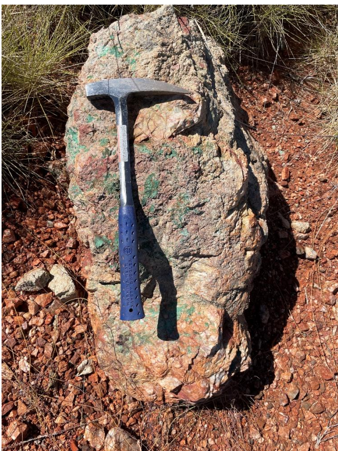
Images 1 – 4 (inclusive): Rock samples collected from the Callawa tenement. Malachite staining is very apparent from the green staining on the faces of the rocks. Hammer has been used for scale.
