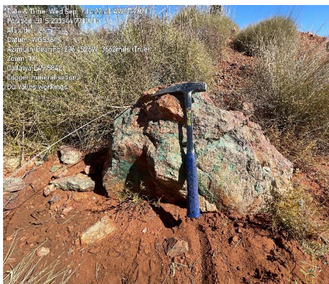
Images 1 – 4 (inclusive): Rock samples collected from the Callawa tenement. Malachite staining is very apparent from the green staining on the faces of the rocks. Hammer has been used for scale.
