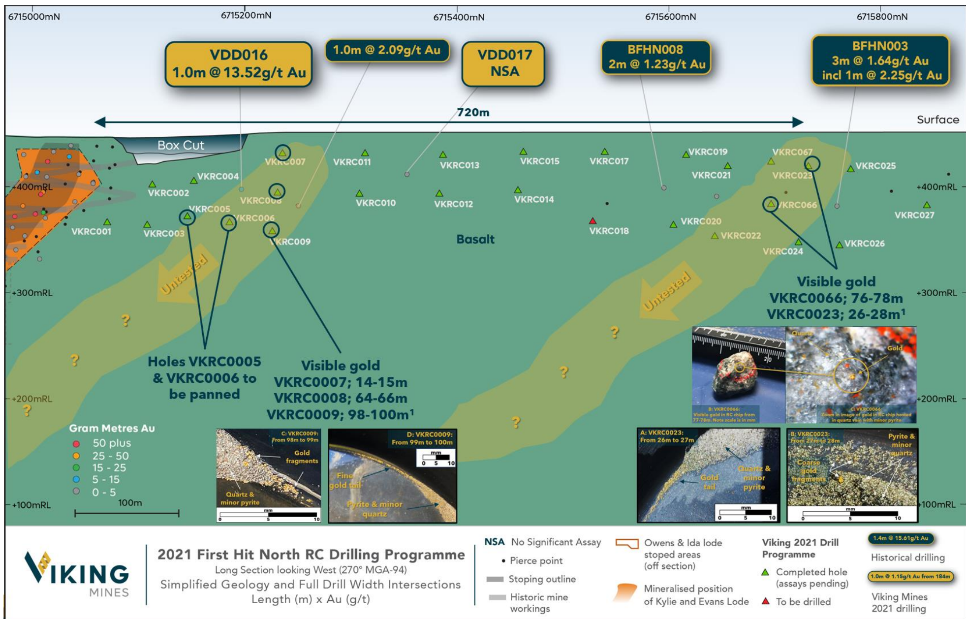
Figure 3: Long section showing location and status of RC drilling programme with completed drillholes shown and location of visible gold observed in RC drill chips. No assays have been received to date for this RC drill programme. The plunge outline of the First Hit shoot and has been superimposed over the areas where visible gold has been seen to illustrate the potential scale and orientation of shoots being explored for. This technique is used by Viking to plan drillholes and determine priorities for further investigation.
