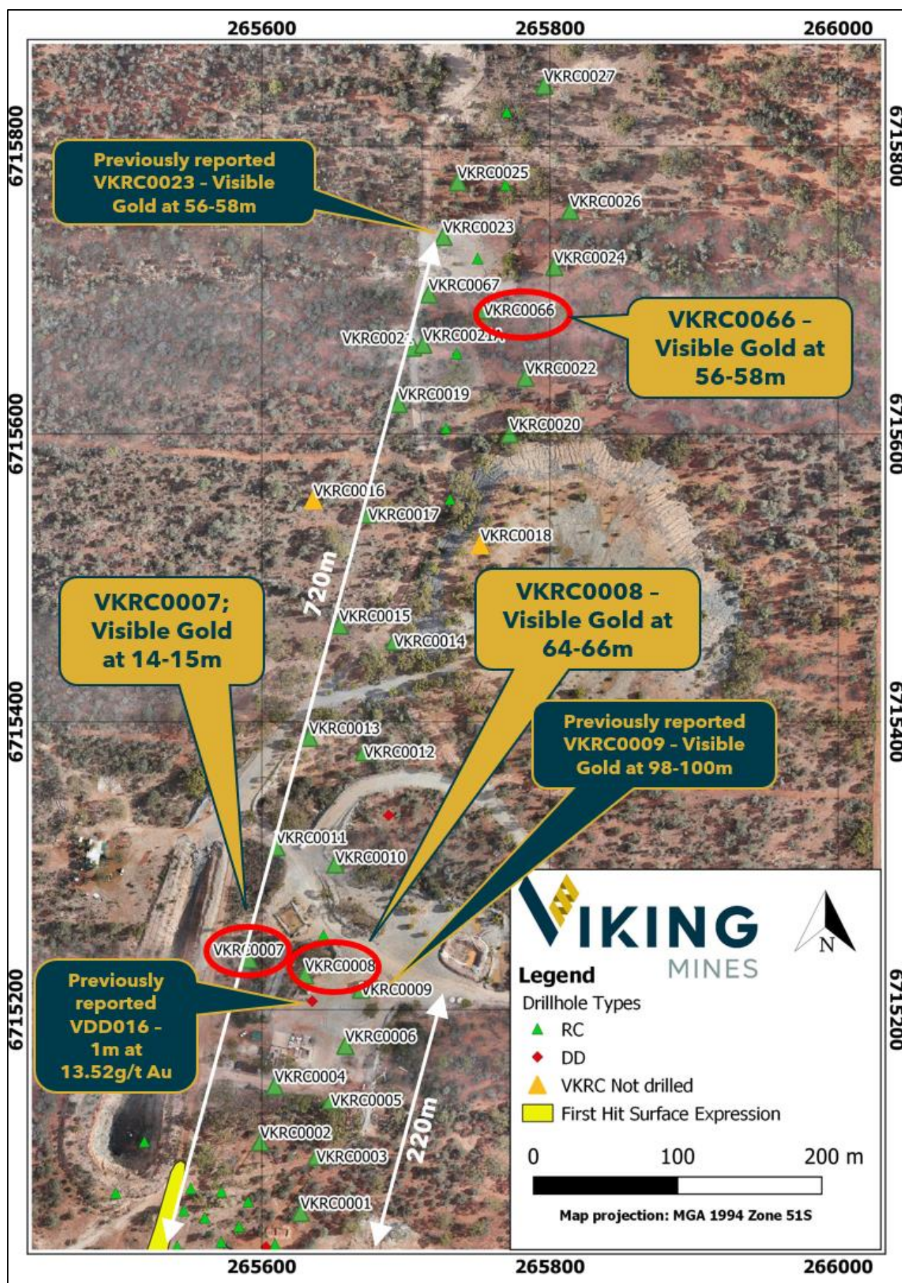
Figure 2: Map showing the location of drilled and undrilled Viking RC drillholes as part of the 2021 RC drill programme. Note location of RC holes with visible gold panned from RC chips. VKRC0007 & VKRC0008 and VKRC0066 220m north and 680m north respectively from the historic First Hit mine workings.
