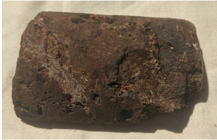
Figure 4: Gronnedal-Ika Sample (IVT 21 – 4) carbonatite, magnetite with 176 ppm Europium from 2.8m. (203.8 ppm \text{Eu}_2\text{O}_3 )
