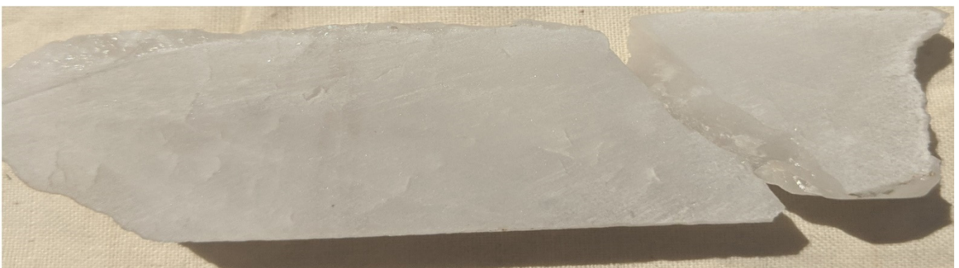
Figure 2: 99.7% SiO 2 in Sample IVT-21-5 of Quartz from 42.18m
