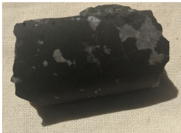
Figure 3: Sample (IVT 21 - 1) magnetite from 71.73ms with 3670 ppm Niobium (5248 ppm Nb 2 O 5 )
