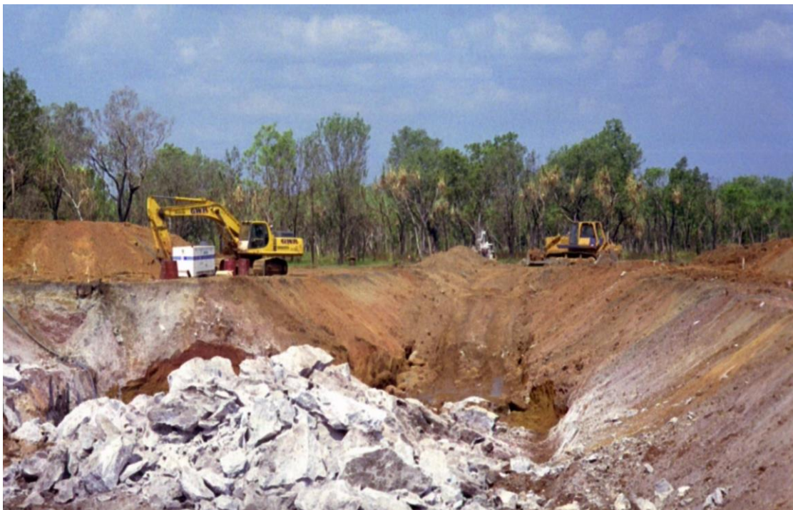
Figure 4 Test mining of magnesium at Winchester during the wet season (after blasting Level 0)
