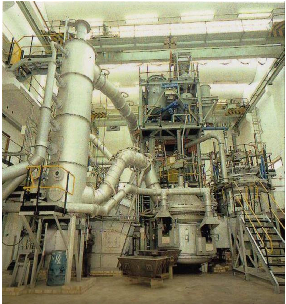
Figure 6 Magnesium plant which produced pure Winchester Mg - condenser (left), arc furnace (right)
