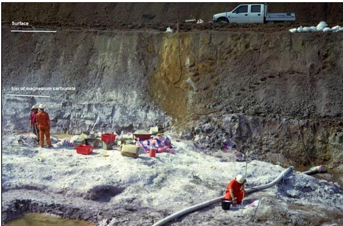
Figure 5 Test mining of magnesium at Winchester during the wet season (preparing to blast Level -1)
