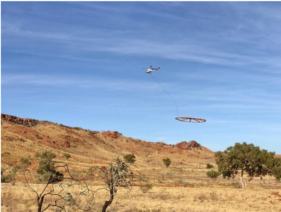
Figure 1: NRG Xcite helicopter EM system flying at Trek Metals' Pincunah Project earlier this month
