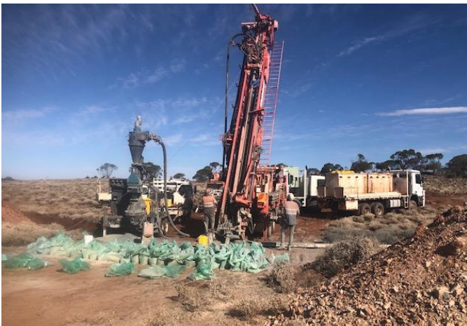
Figure 1: Multipurpose reverse circulation and diamond core rig drilling at Burbanks South
