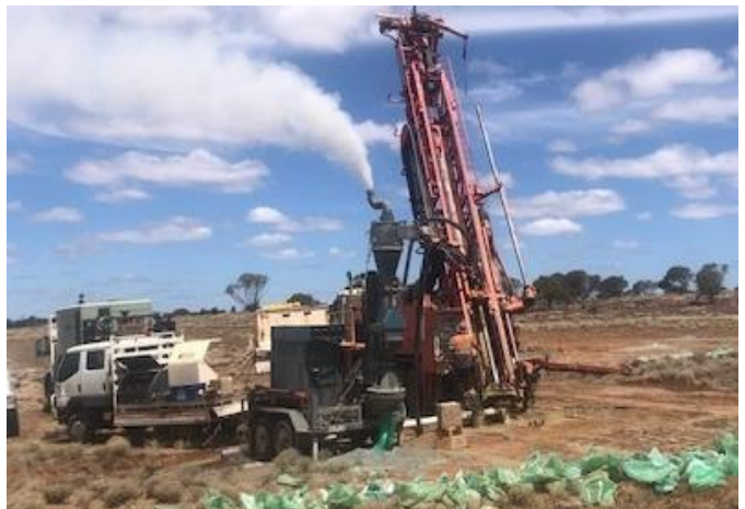
Figure 1: Multipurpose reverse circulation and diamond core rig drilling at Burbanks South
