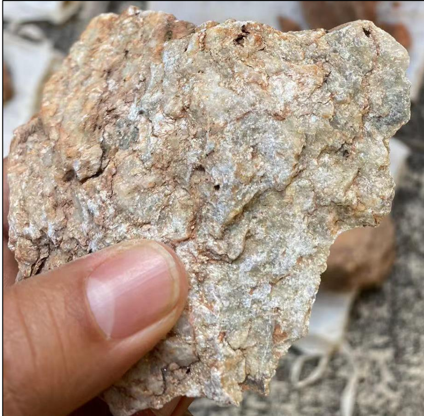
Figure 3: Close look-up of Sample JC001, ~ 40% spodumene by visual estimation (to be confirmed by laboratory analysis)
