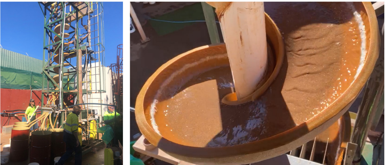
Figure 22: Gravity spirals set-up for the processing of the deslimed and screen material (left) & close-up of the gravity spiral in the early phases of the process (right).
