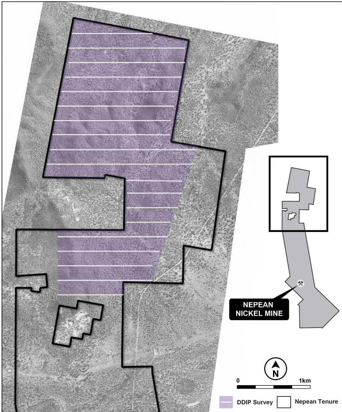
Figure 1 – Map showing location and survey lines of the ground IP survey underway in the north of the Nepean Project
