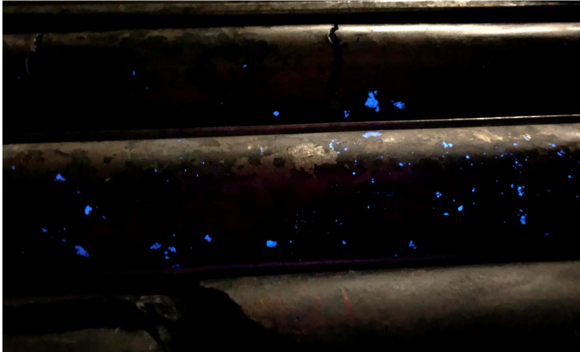
Figure One | Photo of scheelite glowing blue under short wave ultraviolet light in drill core at 120.2 m in ML339M
