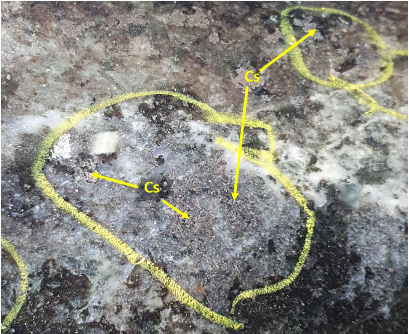
Figure Three | Photo of coarse grained cassiterite (marked as Cs in the yellow circles on the drill core) at 117.3 m in ML339M
