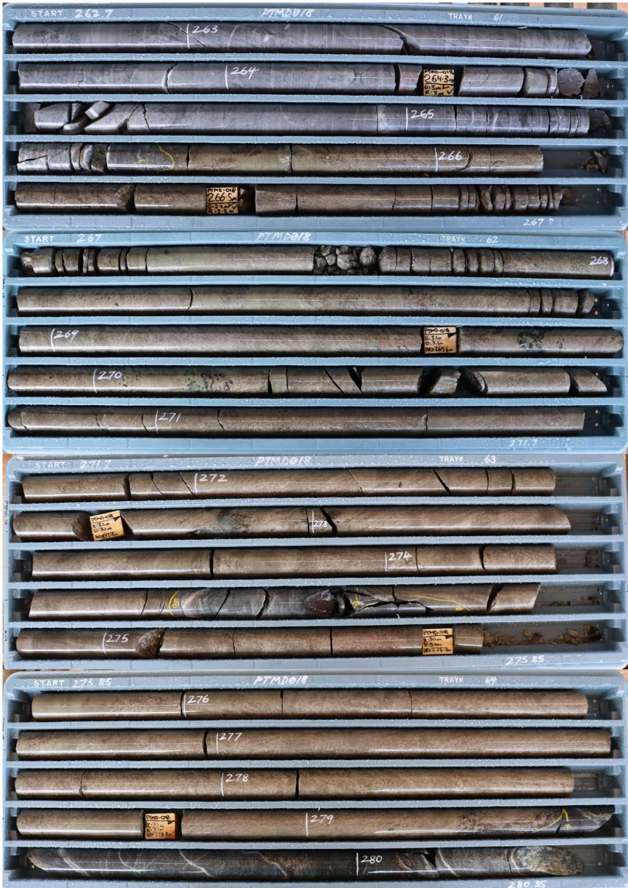
FIGURE 1: VISUAL MASSIVE SULPHIDES IN HOLE PTMD018 FROM 265.5M
