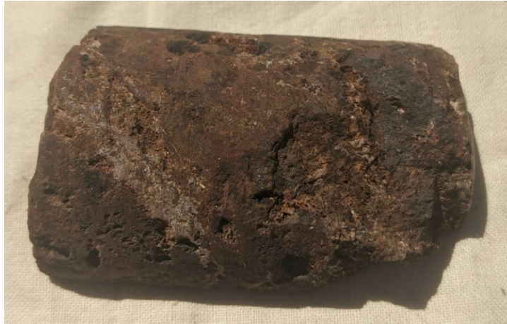
Figure 4: Gronnedal-Ika Sample (IVT 21 – 4) carbonatite, magnetite with assay results returning 203.8 ppm \text{Eu}_2\text{O}_3 and 1,245 ppm \text{Pr}_2\text{O}_3 from 2.8m
