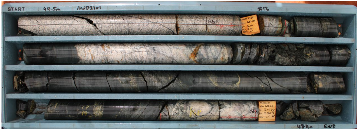
Image 3 | NWD2101: 46m to 48m; 2m @ 1.5% Cu, 0.2 g/t Au and 5.8 g/t Ag
