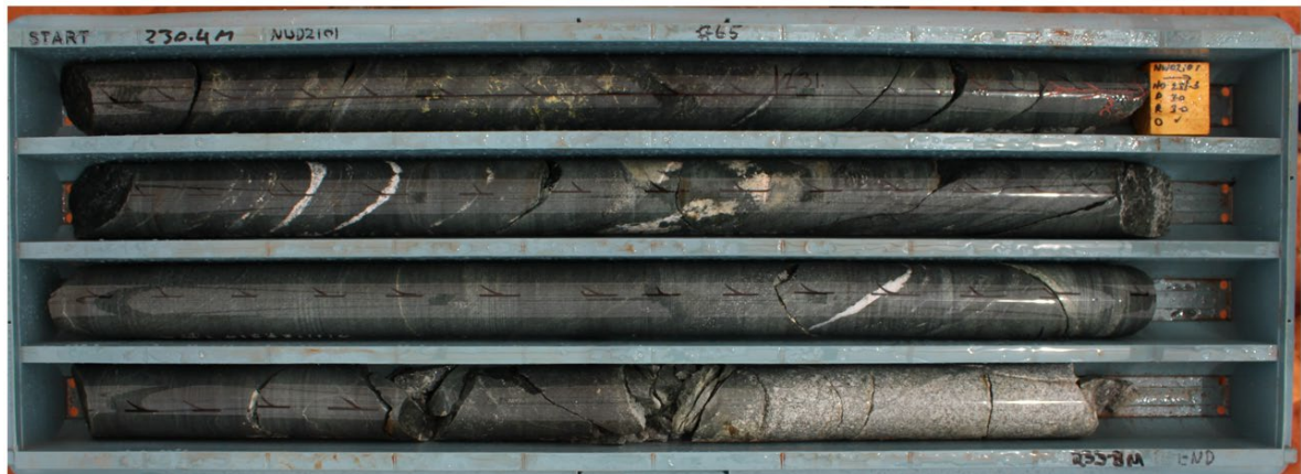
Image 6 | NWD2101: 229m to 231m; 2m @ 3.2% Cu, 0.6 g/t Au and 4.9 g/t Ag
