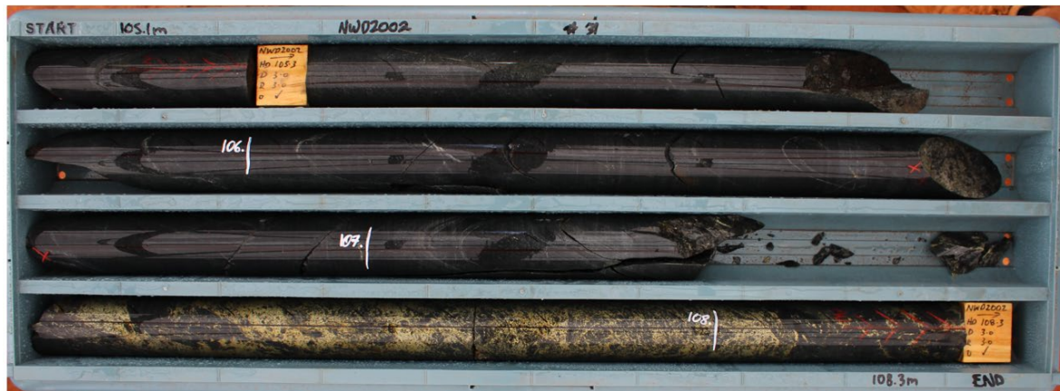
Image 1 | NWD2002: 64m to 66m; 2.0m @ 1.0% Cu, 0.2 g/t Au and 2.0 g/t Ag
