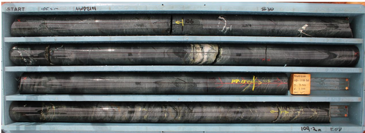
Image 3 | NWD2101: 46m to 48m; 2m @ 1.5% Cu, 0.2 g/t Au and 5.8 g/t Ag
