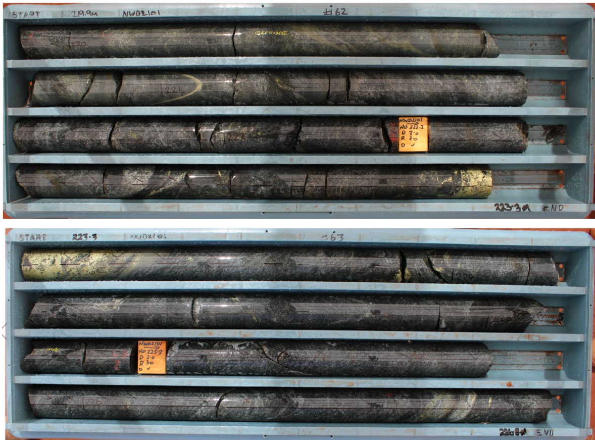
Image 5 | NWD2101: 222m to 224m; 2m @ 3.9% Cu, 0.8 g/t Au and 6.1 g/t Ag
