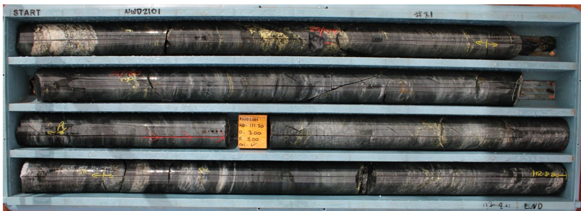
Image 4 | NWD2101: 108m to 110m; 2m @ 1.8% Cu, 0.4 g/t Au and 3.6 g/t Ag
