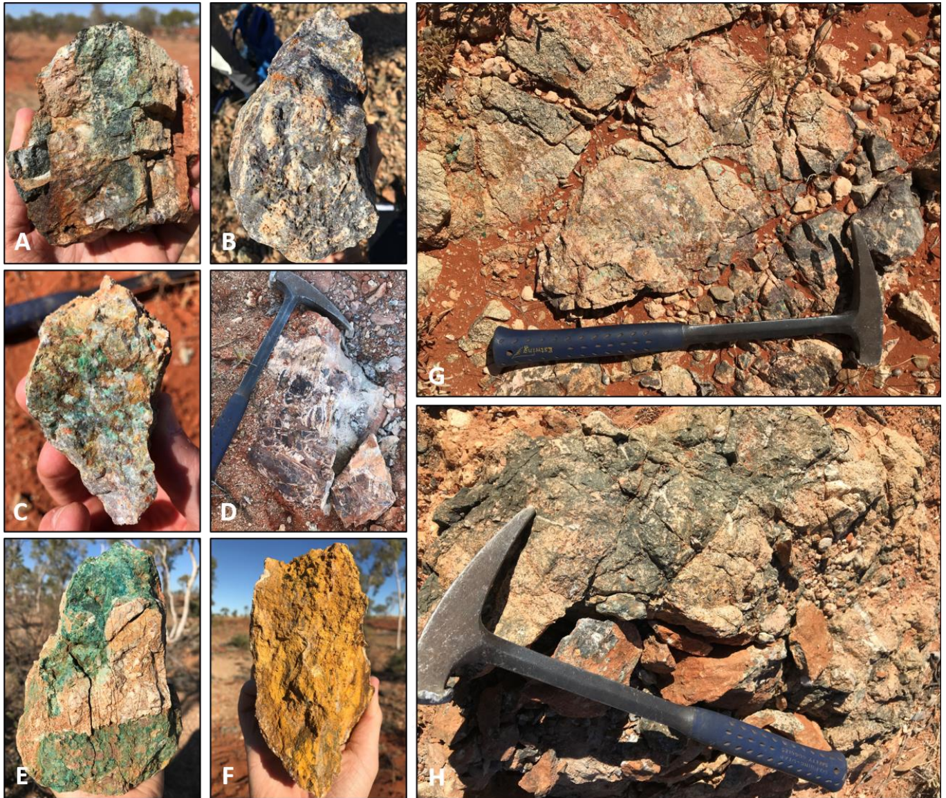
Figure 3 Selection of Ningaloo rock chips including: A) JE0094 with 0.36g/t Au + 1.42% Cu + 957ppm Bi; B) JE0105 with 0.19% Cu; C) JE0098 with 1.27% Cu; D) JE0103 with 0.46% Cu; E) JE0107 with 9.65% Cu + 2.93g/t Ag; F) JE0108 with 0.16% Cu; G) JE0096 with 1.28% Cu; and H) JE0110 with 0.19% Cu. This photo collage of samples first appears in ASX announcement dated 3 June 2021.
