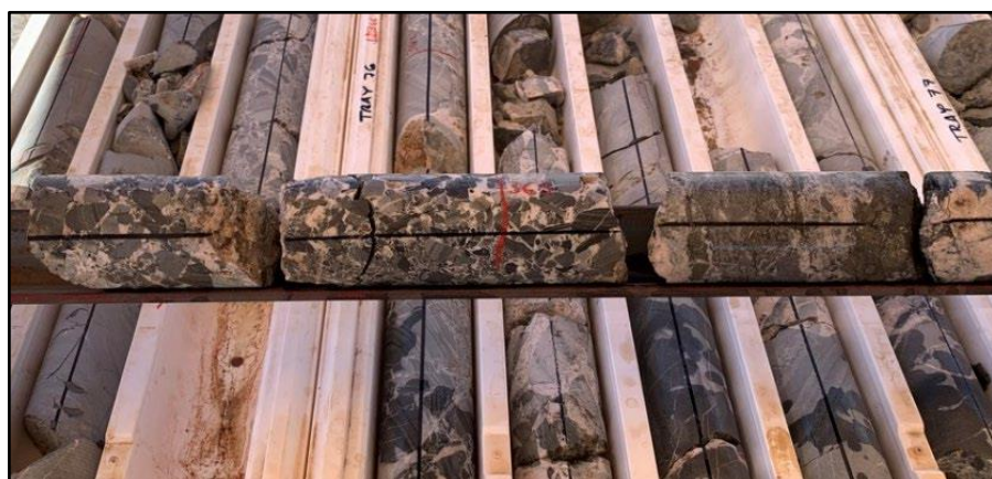
Above: NQ2 core from diamond drillhole 20ALDD0003 showing typical brecciation at approximately 365m downhole
