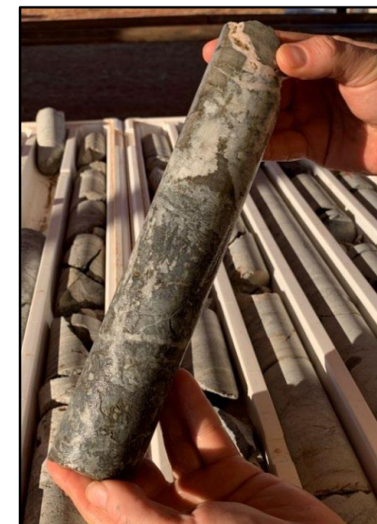
Above: NQ2 core from diamond drillhole 20ALDD0003 showing typical brecciation at approximately 365m downhole
