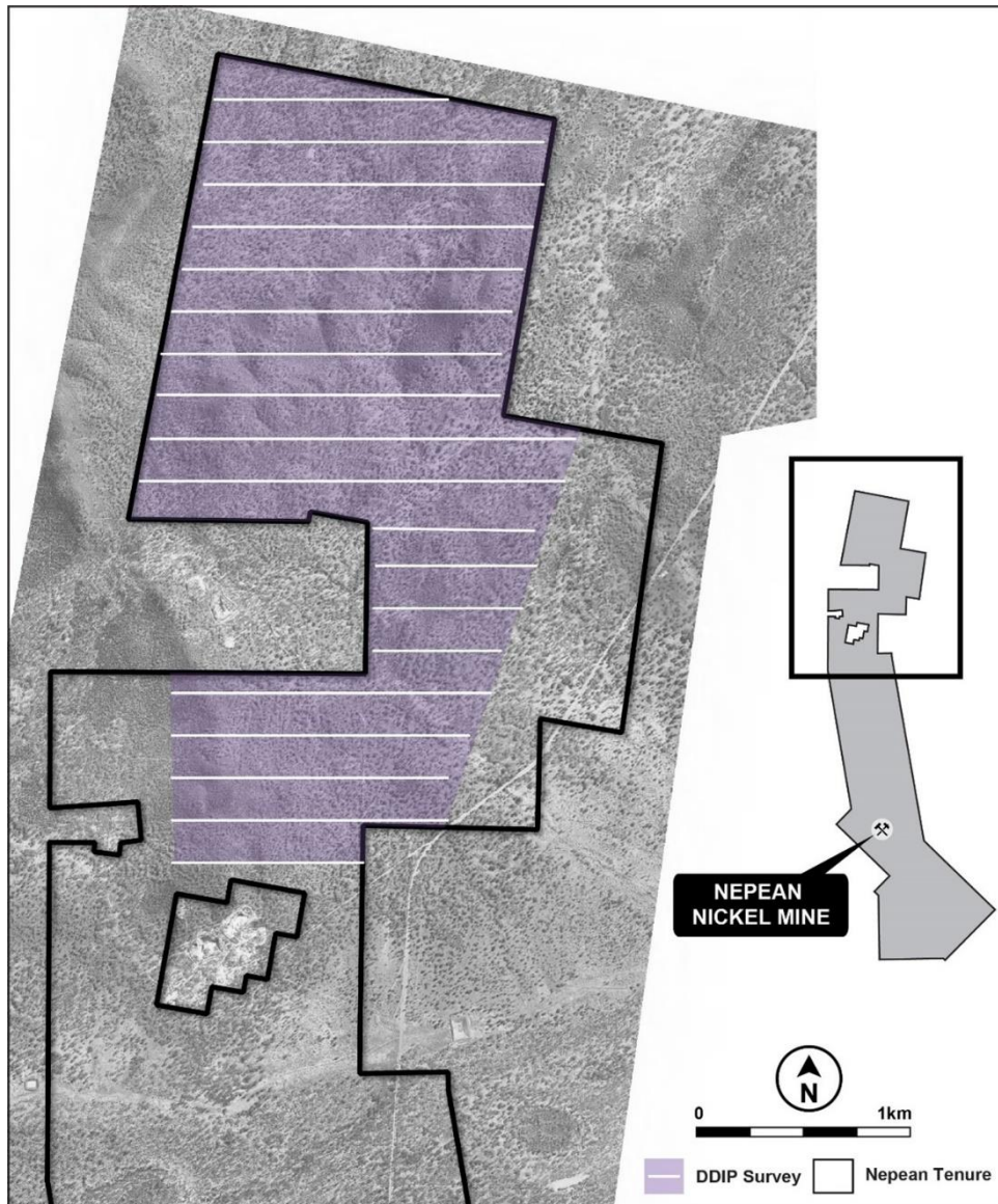
Figure 2 – Map showing location and survey lines of the ground IP survey underway in the north of the Nepean Project. To-date the northern five lines have been surveyed
