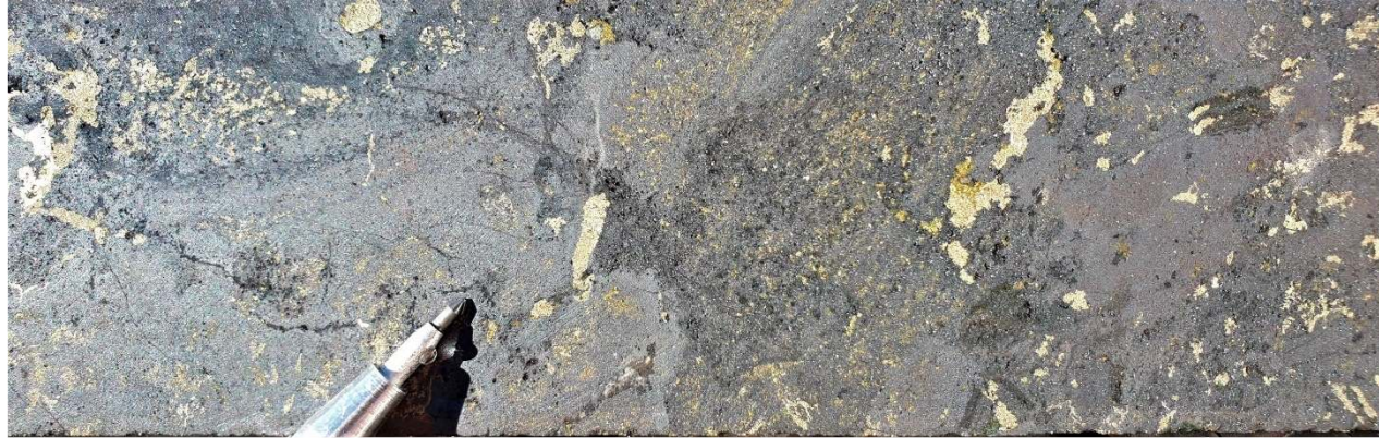
VUD0019 - 1411.2m. Disseminated chalcopyrite and pyrite mineralisation in hematite breccia. NQ2 ½ core.
