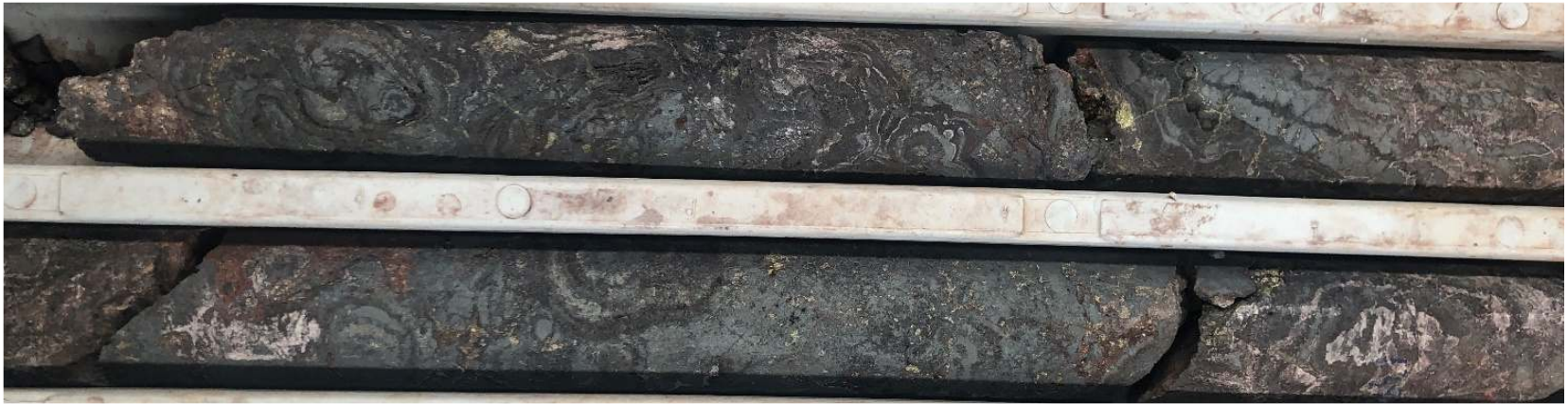
VUD0018 - 1387m. Mineralised colloform massive hematite breccia. NQ2 core.
